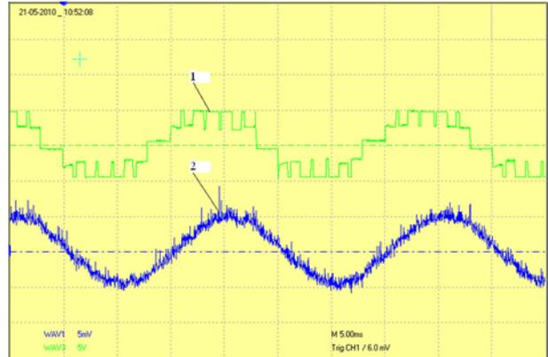
Fig. 9: Experimental results: 1 – output voltage  $U_{out}$ ; 2 – output current  $I_{out}$  with  $U_{max} = 0.95$
