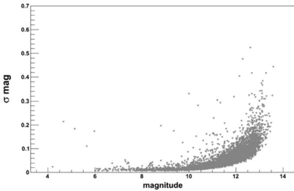
Fig. 2: Precision of star brightness measurements from standard photometry, for 200 s exposures (20 coadded frames) from the “Pi of the Sky” prototype in the Las Campanas Observatory in Chile
