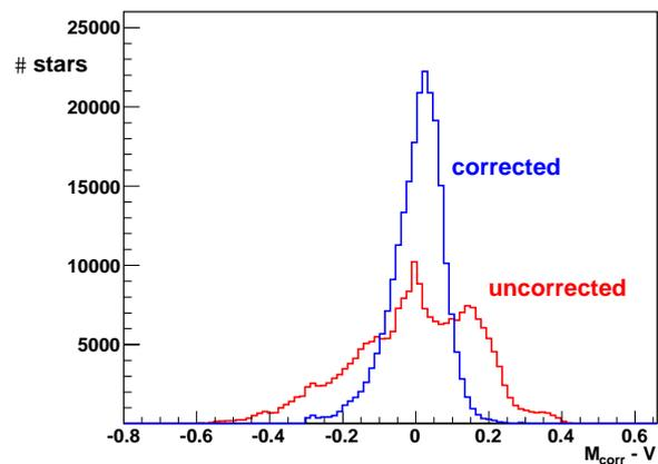
Fig. 5: Distribution of the difference between the measured reference star magnitude and the catalogue *V* magnitude before (red) and after (blue) spectral correction
