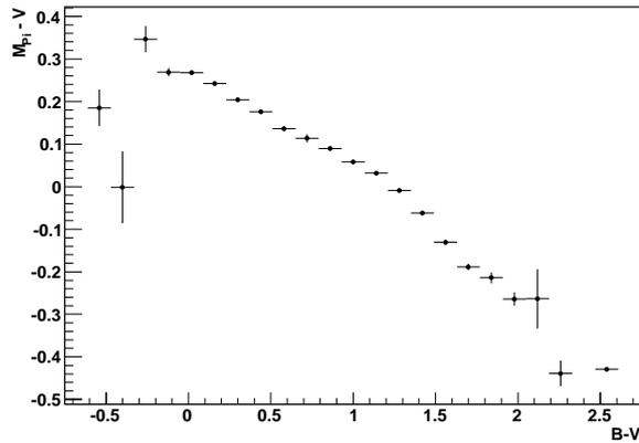
Fig. 4: Average difference between the “Pi of the Sky” magnitude  $M_{Pi}$  and the catalogue *V* magnitude for the reference stars, as a function of the spectral type given by  $B - V$
