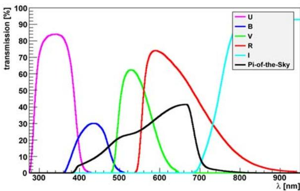
Fig. 3: Spectral sensitivity of the “Pi of the Sky” detector, as resulting from the CCD sensitivity and IR+UV filter transmission, compared to the transmission curves of standard photometric filters
