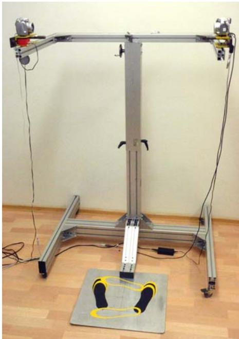
Fig. 6: The two-arm stand with fixed cameras and laser collimators
