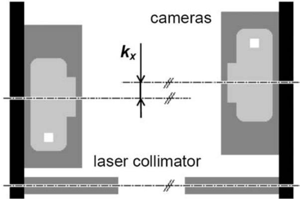
Fig. 5: Displacement of optical axes
