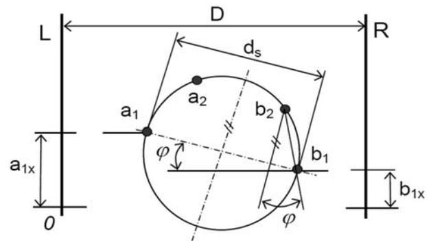
Fig. 3: Geometry used for measuring the head position
