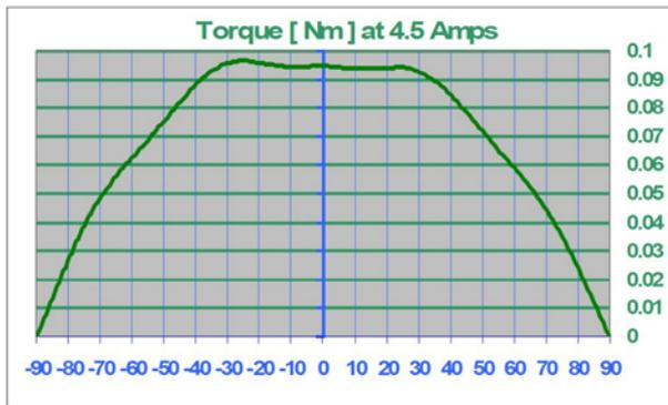
Fig. 3: Torque versus electric angle diagram
