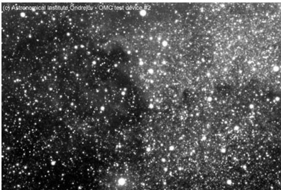
Fig. 2: Test image provided by the OMC Test Device operated at the Ondrejov Observatory (FOV 6 \times 7 deg, lim mag 15.5, pixel size 18 arcsec identical with the real OMC camera)
