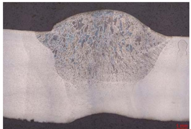
Figure 7: Sample B3 — capping layer, short arc 145 A
