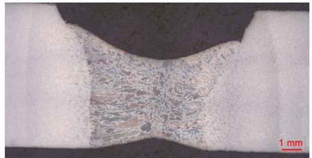
Figure 6: Sample B3 — root weld, short arc 130 A
