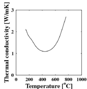
Fig. 1b: Dependence of the thermal conductivity of Penly concrete on temperature
