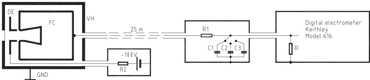
Fig. 2: Block scheme of the Faraday cup including the electrical measuring chain: FC – Faraday cup, DE – decelerating electrode, VH – vacuum housing, R1 –  $0.2\text{ M}\Omega$ , R2 –  $0.5\text{ M}\Omega$ , R – electrometer input range resistor  $10^5 - 10^{11}\Omega$ , C1 –  $4.7\mu\text{F}$ , C2 –  $0.1\mu\text{F}$ , C3 –  $1\text{nF}$
