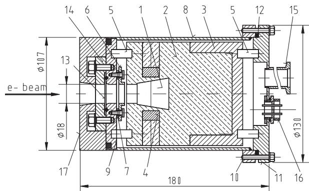
Fig. 1: Assembly drawing of the Faraday cup in the vacuum housing: 1 – cavity, 2 – graphite cup, 3 – steel stopper, 4 – permanent magnets, 5 – ceramic insulators, 6 – decelerating electrode, 7 – insulators, 8 – cylindrical part of the vacuum housing, 9 – housing bottom, 10 – collar, 11 – rear flange, 12 – rubber gasket, 13 – Al foil entry window, 14 – front flange, 15 – pumping sleeve, 16 – vacuum 4-lead bushing, 17 – Al front shielding
