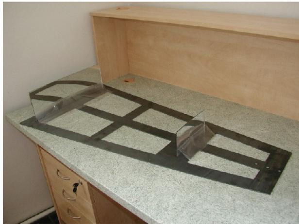
FIGURE 4. Two parabolic strips of lengths 20 and 40 cm; for the proof-of-principle experiment, the 40 cm strip was used.
