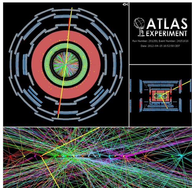
FIGURE 1. Display of a  $Z \rightarrow \mu^+ \mu^-$  candidate event recorded by the ATLAS detector with 25 additional pp collision vertices reconstructed in the tracking detectors.
