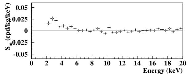
FIGURE 2. Energy distribution of the modulation amplitudes  $S_m$  for the total cumulative exposure 1.17 t yr obtained by maximum likelihood analysis. The energy bin is 0.5 keV. A clear modulation is present in the lowest energy region, while  $S_m$  values compatible with zero are present just above. In fact, the  $S_m$  values in the  $(6 \div 20)$  keV energy interval have random fluctuations around zero with  $\chi^2$  equal to 27.5 for 28 degrees of freedom [9, 10].
