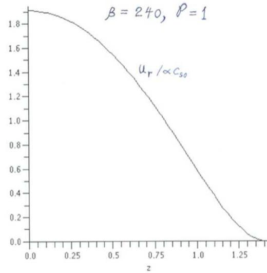
FIGURE 3. Distribution of the radial velocity over the thickness in the stationary accretion disk with a large scale poloidal magnetic field.
