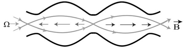
FIGURE 4. Qualitative picture of jet confinement by magneto-torsional oscillations.
