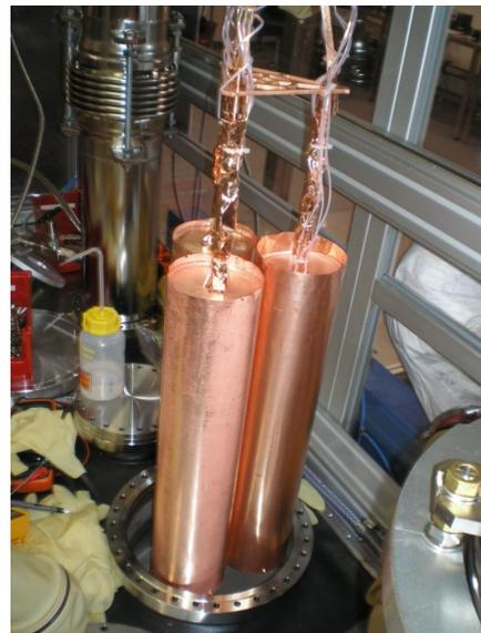
FIGURE 1. Strings of detectors inside the minishrouds.
