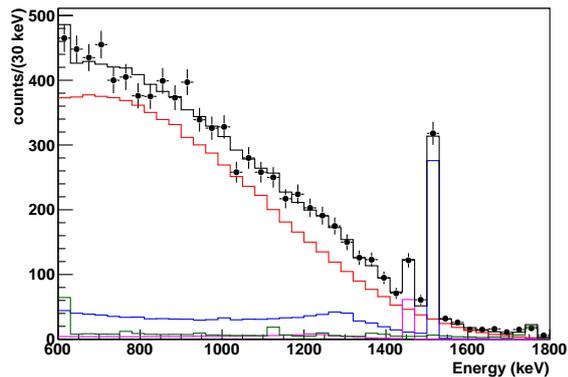
FIGURE 5. Zoom of the  $2\nu\beta\beta$  region, and component decomposition ( $2\nu\beta\beta$ ,  $^{42}\text{K}$ ,  $^{214}\text{Bi}$ ,  $^{40}\text{K}$ ; black line: component sum, black dots: data).
