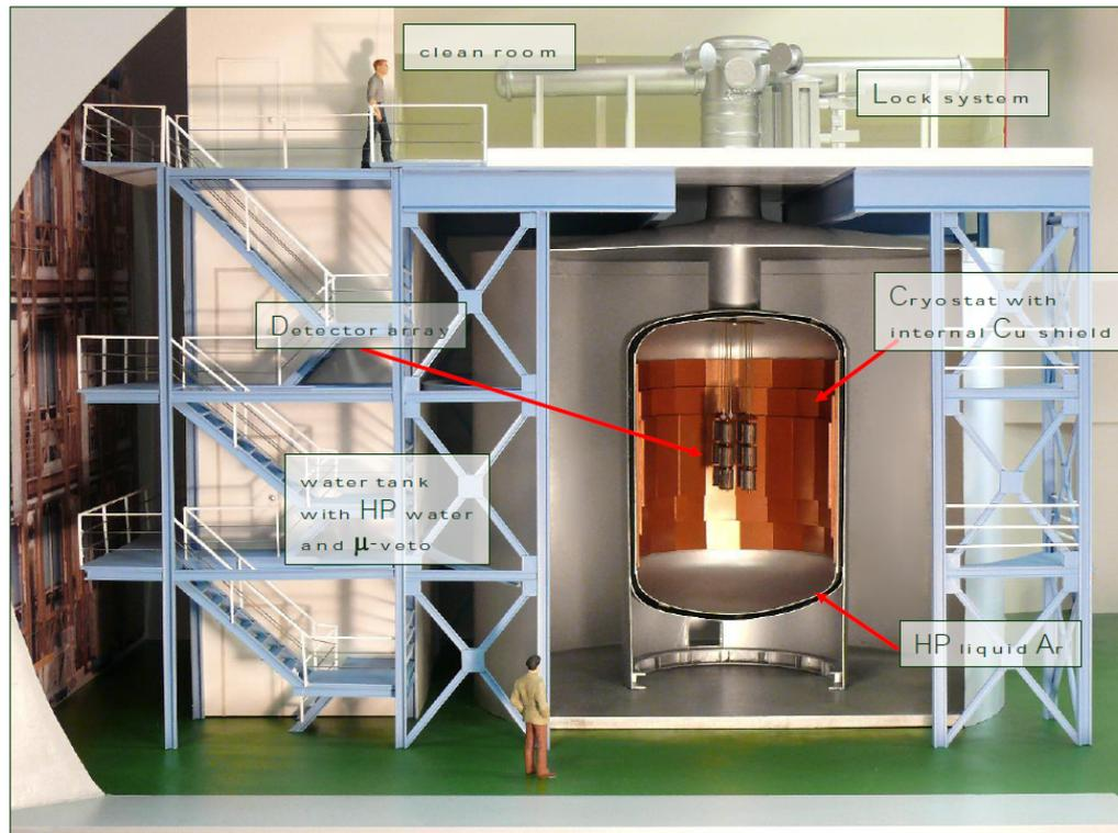
FIGURE 2. Sketch of the GERDA experiment, which is located in the Laboratori Nazionali del Gran Sasso.
