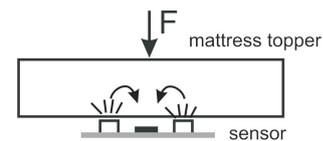
FIGURE 4. Sensor under a mattress.
