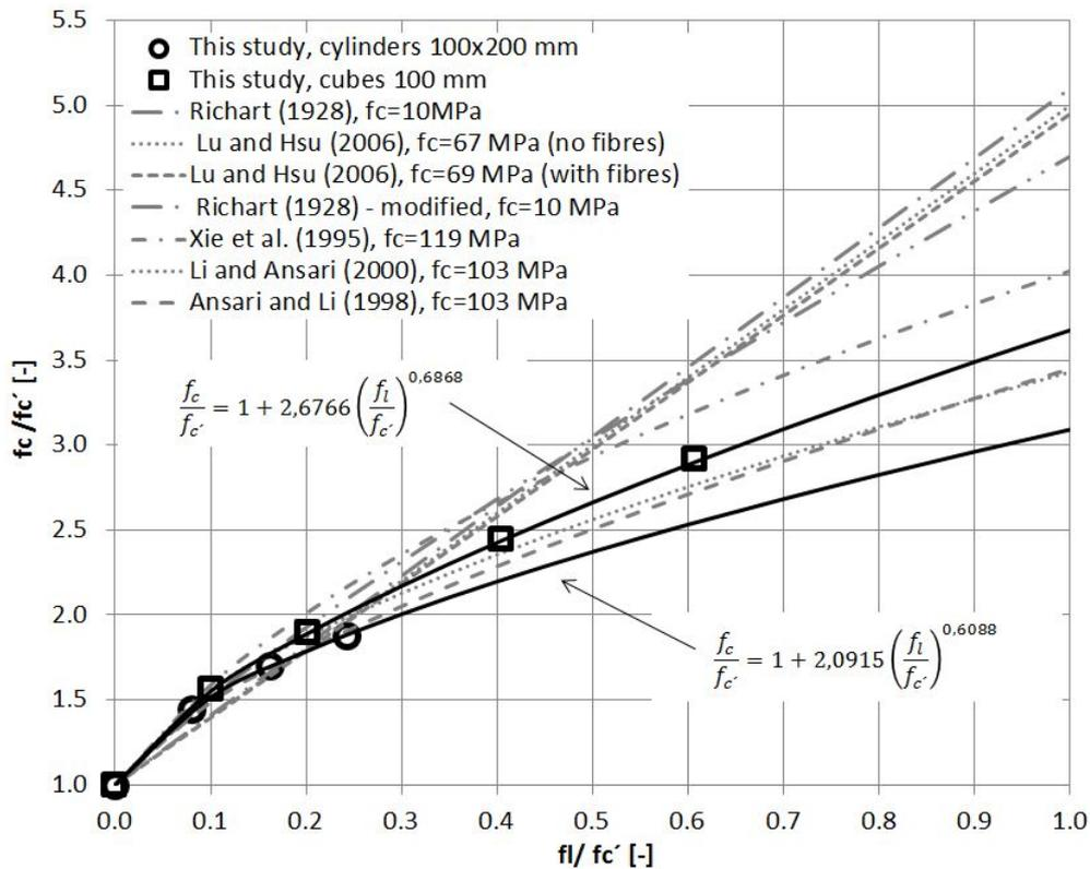
FIGURE 3. Development of triaxial compressive strength.
