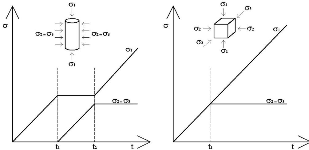
FIGURE 1. Testing procedure for UHPC cylinders and cubes.
