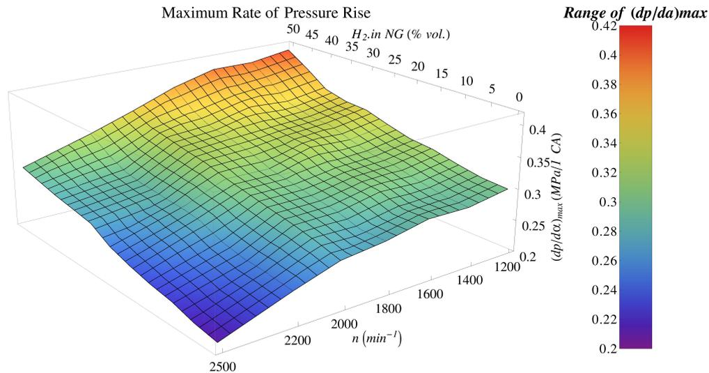
FIGURE 4. Course of values representing the rate of pressure rise  $\left(\frac{dp}{d\alpha}\right)_{\max}$  depending on the revolutions ( $n$ ) for various compositions of mixtures ( $H_2$  in NG) of natural gas and hydrogen (full load, stoichiometric air-fuel mixture, ignition advance  $33.5^\circ$  CA BTDC).
