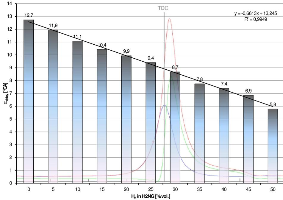
FIGURE 1. Delay of ignition values ( $\alpha_{\text{delay}}$ ) for various mixture compositions (H<sub>2</sub>NG0–H<sub>2</sub>NG50), with indicated line equation and coefficient of reliability (full load, revolutions 1500 min<sup>-1</sup>, advance of ignition 33.5° CA BTDC, stoichiometric air-fuel mixture).
