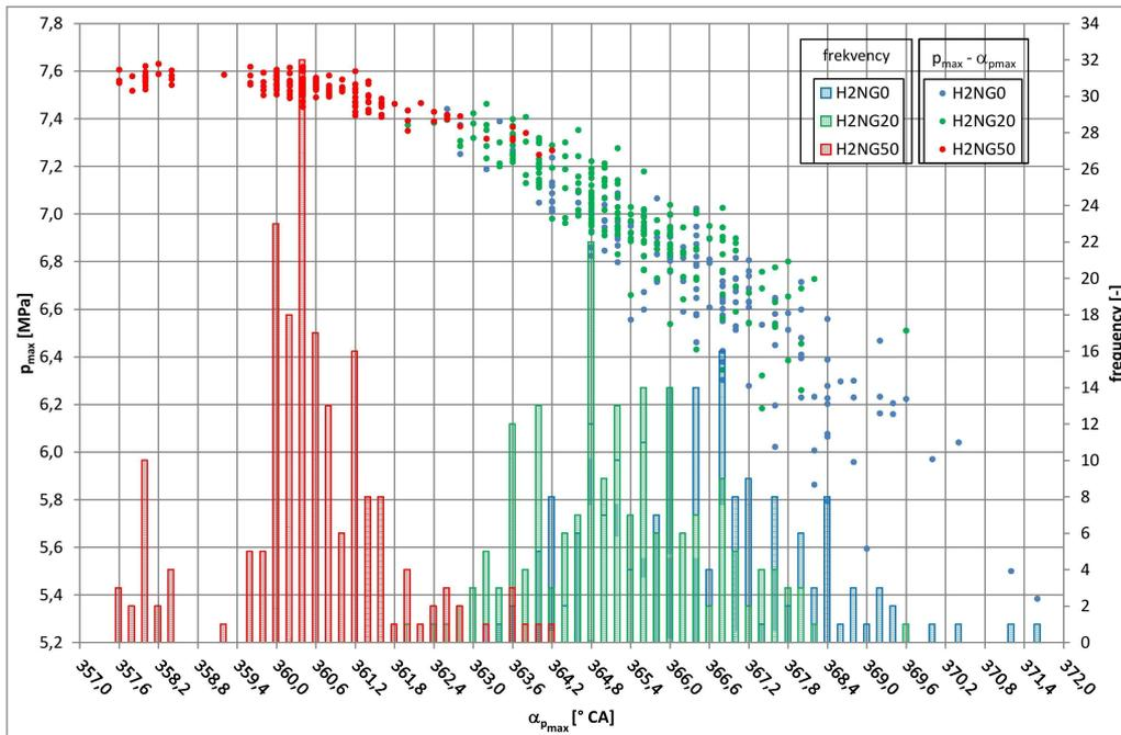
FIGURE 2. Values of maximum pressure ( $p_{\max}$ ) in the combustion chamber and their position ( $\alpha_{p_{\max}}$ ), indicating the frequency of repetitions (full load, revolutions  $1500 \text{ min}^{-1}$ , advance of ignition  $33.5^\circ \text{ CA BTDC}$ , stoichiometric air-fuel mixture).
