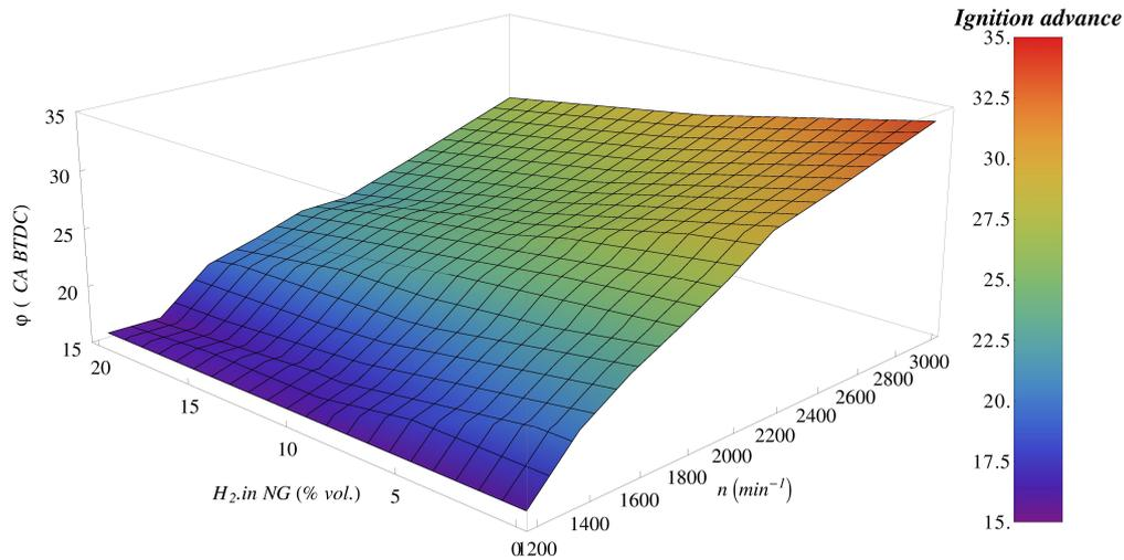
FIGURE 3. Courses representing the optimum angle of spark advance ( $\varphi$ ) for mixtures of various compositions ( $H_2$  in NG), depending on the revolutions ( $n$ ) of the combustion engine (full load, stoichiometric air-fuel mixture).
