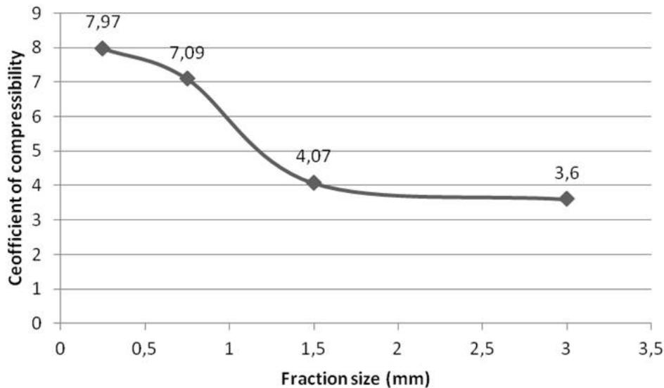
FIGURE 6. Resulting character of approximated coefficient of compressibility values, depending on the mean of the fraction size ranges.
