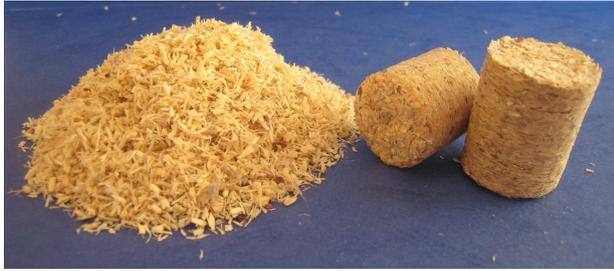
FIGURE 1. Particulate matter from wood mass suitable for direct compression.
