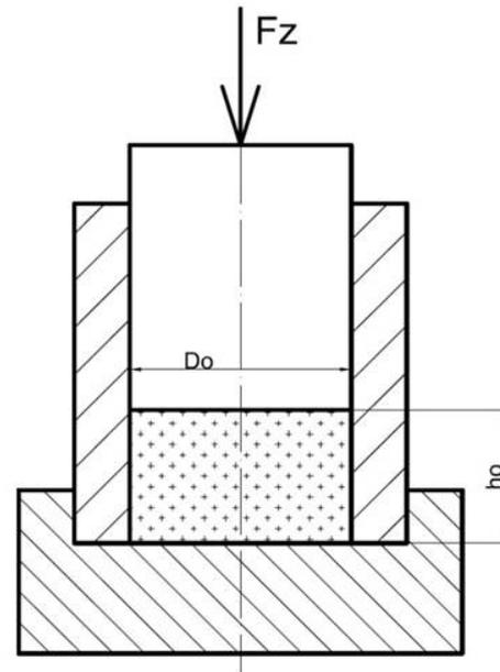
FIGURE 2. Scheme of the function of an oedometer.
