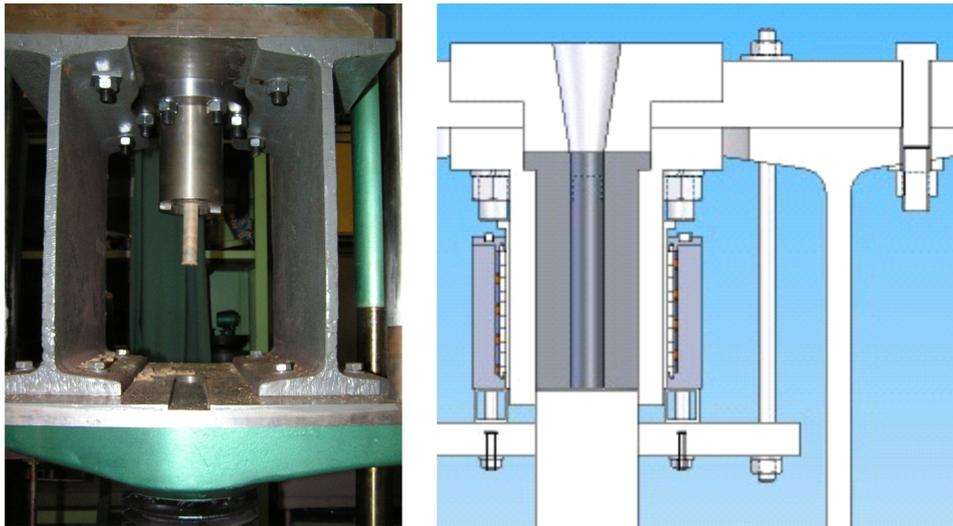
FIGURE 3. The oedometer used in the experiment.
