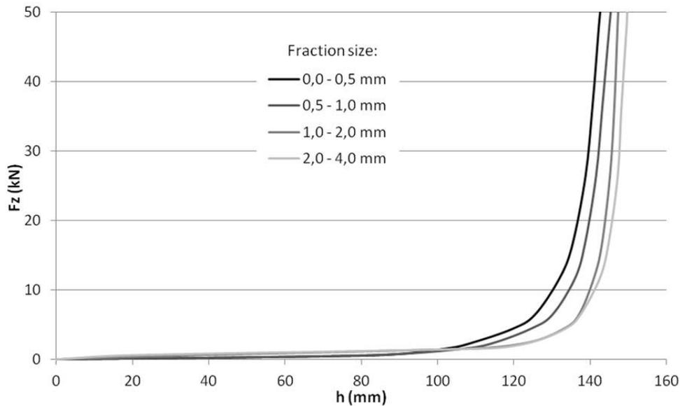
FIGURE 4. Compressibility curve of pine sawdust of various fraction sizes (relative moisture 15,5%; pressing temperature 20°C).
