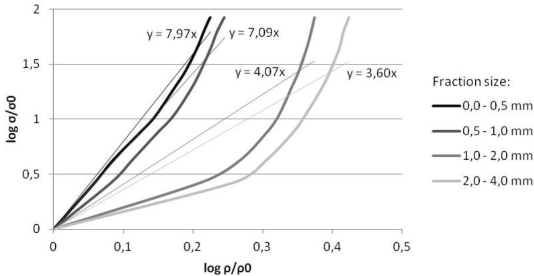
FIGURE 5. Dependence of  $\log \frac{\sigma}{\sigma_0}$  on  $\log \frac{\rho}{\rho_0}$  and linear approximation.
