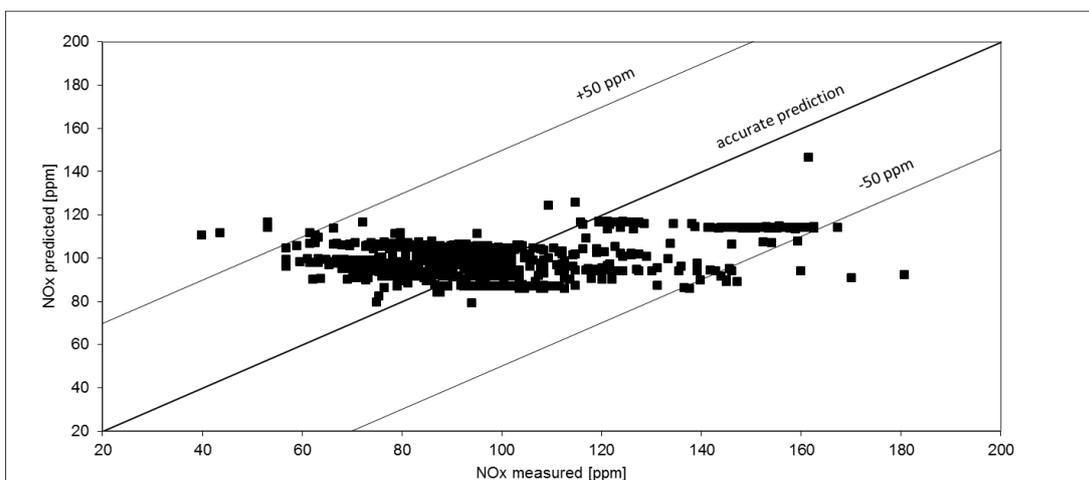
FIGURE 4. NO<sub>x</sub> prediction reliability using Pohl's method with incorporated temperature and excess oxygen dependency.
