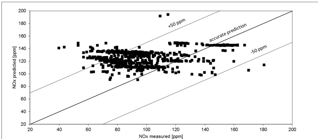
FIGURE 3. NO<sub>x</sub> prediction reliability using Pohl's method with modified constant  $k_1$
