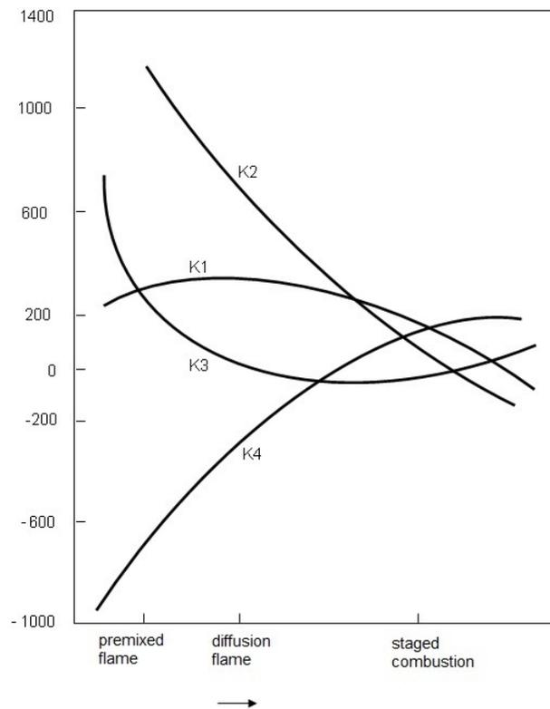
FIGURE 1. Pohl's correlation coefficients for PCC boilers [9].
