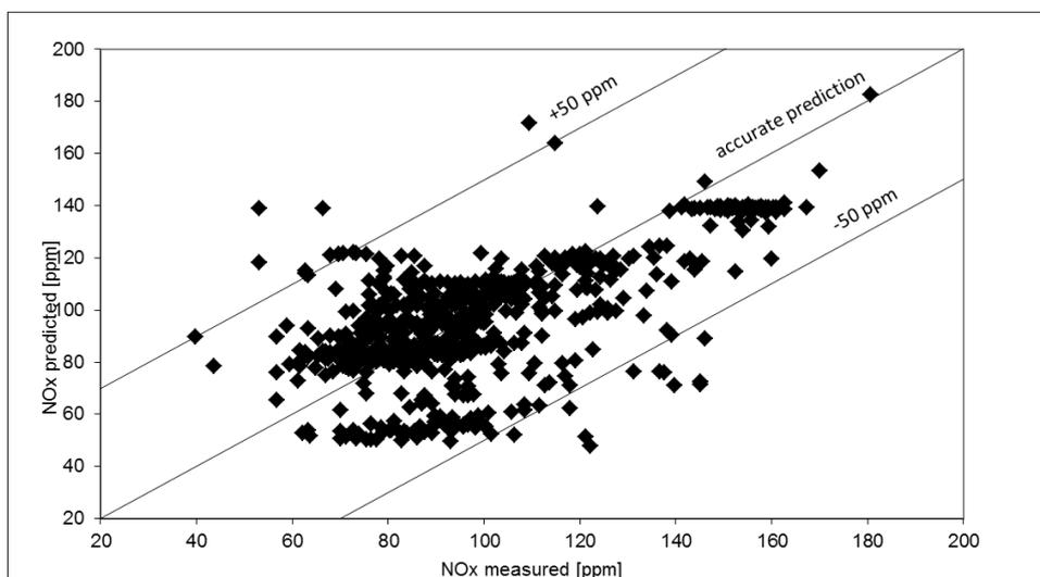
FIGURE 6. NO<sub>x</sub> prediction reliability using Ibler's method with optimized constants.
