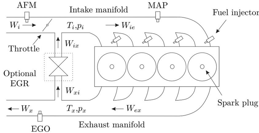
FIGURE 3. Simplified schematics of an SI engine.
