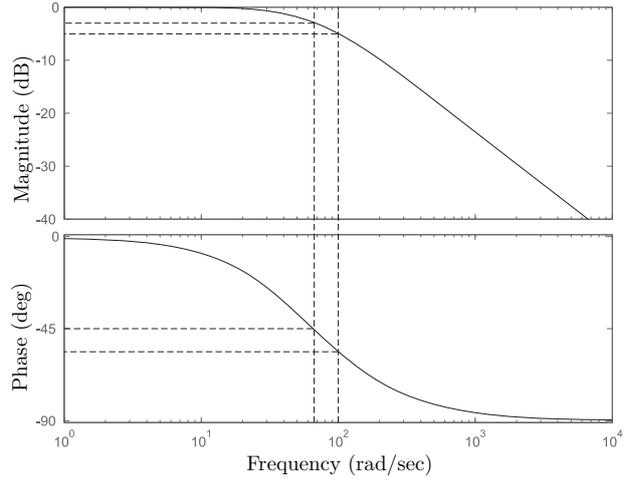
FIGURE 5. Bode diagram for the transfer function  $G(s)$ .
