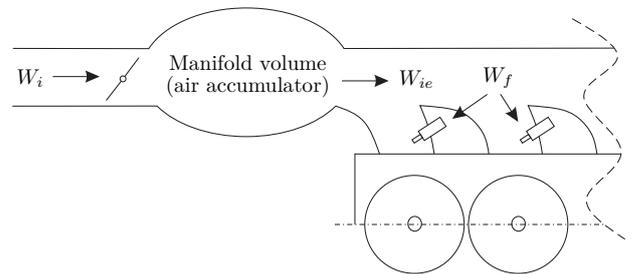
FIGURE 9. Schematic representation of the intake manifold.
