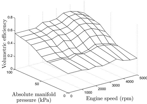
FIGURE 6. Measured volumetric efficiency map.
