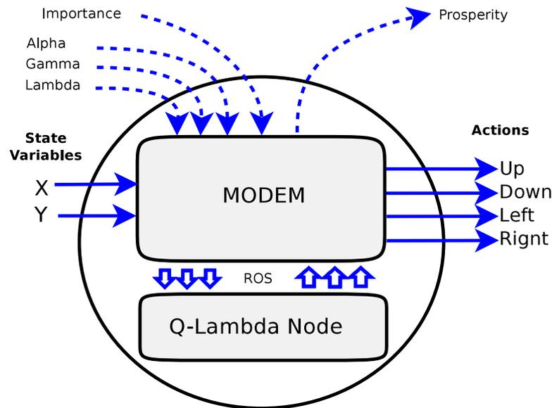
FIGURE 1. A Neural Module with two data inputs, four data outputs and four configuration inputs. The module also contains "Prosperity" output, which provides subjective heuristics defining how well the module performs in the current architecture during the current simulation. Here, a modem serves as a communication interface between the NengoROS simulator and an external ROS node, which implements a given algorithm/functionality.
