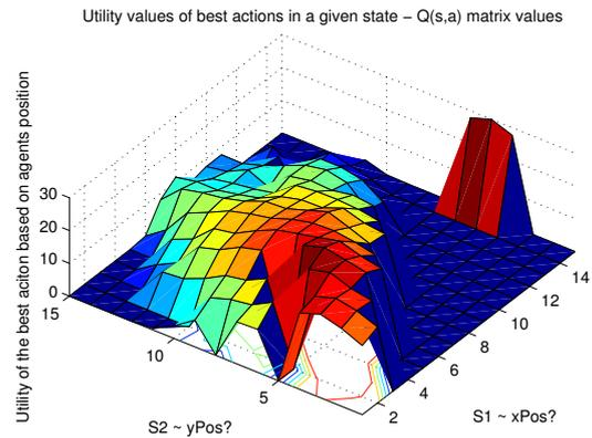
(b) Knowledge of the selected agent found by SORGA – Ind1. The Q-Lambda Module has swapped axes and the value of the S2 variable is computed as follows:  $S2 = X + 0.71Y$ . This causes slower convergence of learning. The “peak” in the graph is caused by connecting the reward output to the S1 input.
