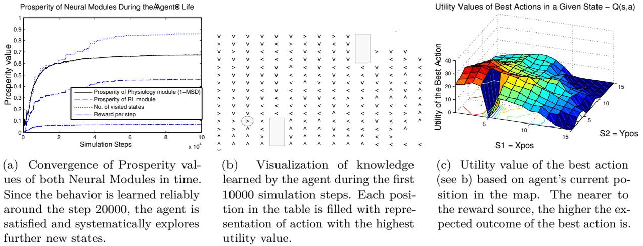
FIGURE 6. Simulation of the hand-designed agent architecture. Each position in b) and c) represents one position in the map. There are two obstacles and one source reward in the environment. b) and c) show the agent's learned knowledge. Greedy ASM selects the action with the highest utility in each state. These actions are shown in b) and their utility is shown in c). Note that the utility values on the Z-axis are rescaled for better visibility.
