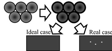
FIGURE 5. The sintering process a) real case (creating closed pores); b) ideal state (without pores).
