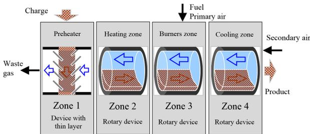
FIGURE 4. Example of the model arrangement of a rotary furnace with preheater and cooler.
