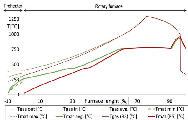
FIGURE 11. Caustic production — comparison of the course of temperatures of a standard operation (reference state) and while using a preheater.
