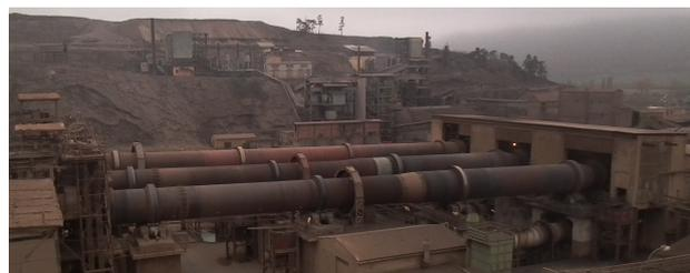
FIGURE 1. Rotary furnaces for magnesite sintering.
