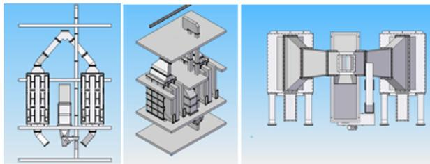
FIGURE 13. Visualisation of preheater based on the principle of thin layer for the rotary furnace No. 2.
