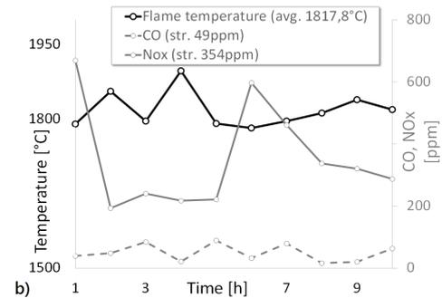
FIGURE 9. Measurement at the sintering regime a) thermal camera — warm head; b) course of temperatures and change of the flue gas composition.
