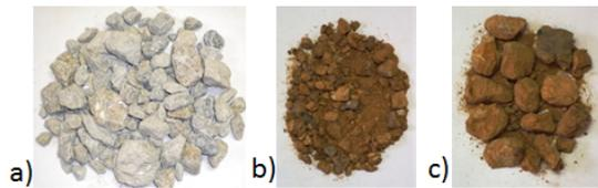
FIGURE 7. Grain size analysis K2 10–40 mm: a) starting raw magnesite material; b) after annealing the granularity samples 31,5 mm maximum; c) after annealing the granularity samples 31,5 mm minimum.
