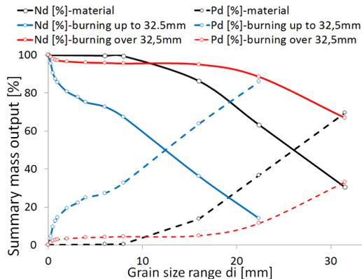
FIGURE 8. Distribution curve of the dependence of summary weight yield from granulometric range — oversize (Nd) a undersize fraction (Pd).
