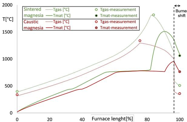
FIGURE 10. Course of material and flue gas temperatures at the calibrated model.
