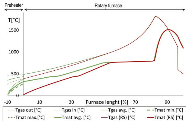
FIGURE 12. Clinker production — comparison of the course of temperatures of a standard operation (reference state) and while using a preheater.
