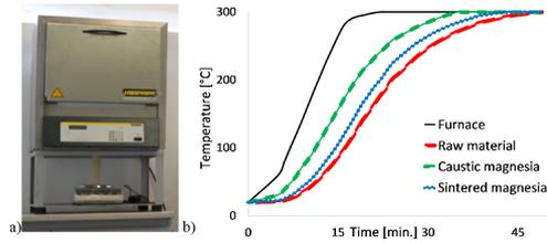
FIGURE 6. Laboratory determination of the spread of heat transfer, a) equipment; b) course of curves.
