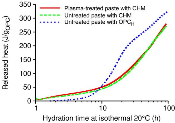
FIGURE 4. Hydration heat of plasma-treated CHM.
