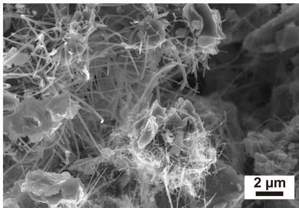
FIGURE 1. SEM image of the cement hybrid material with CNTs synthesized on its surface.
