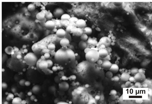
FIGURE 2. SEM image of the Opatovice fly ash.
