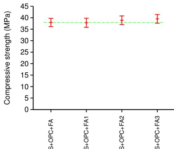
FIGURE 7. Compressive strength of the mortar with untreated and treated FA after 36 days with standard deviation.
