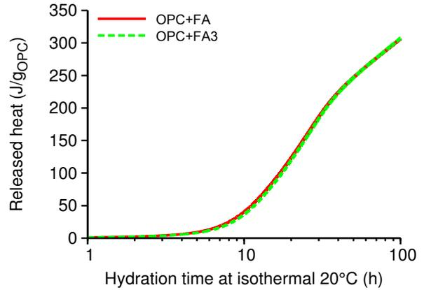
FIGURE 5. Hydration heat of FA and plasma-treated FA3 in cement pastes.
