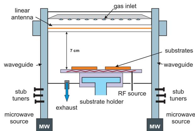
FIGURE 3. Schematic drawing of the pulsed linear antenna microwave plasma deposition system with RF substrate bias.
