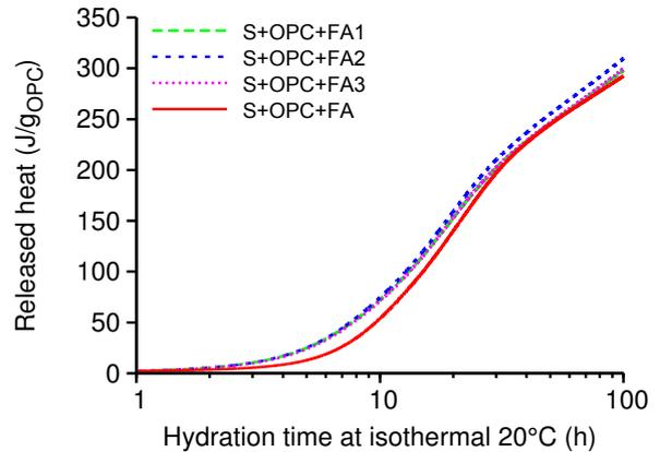
FIGURE 6. Hydration heat of raw FA and plasma-treated FAs in mortars.
