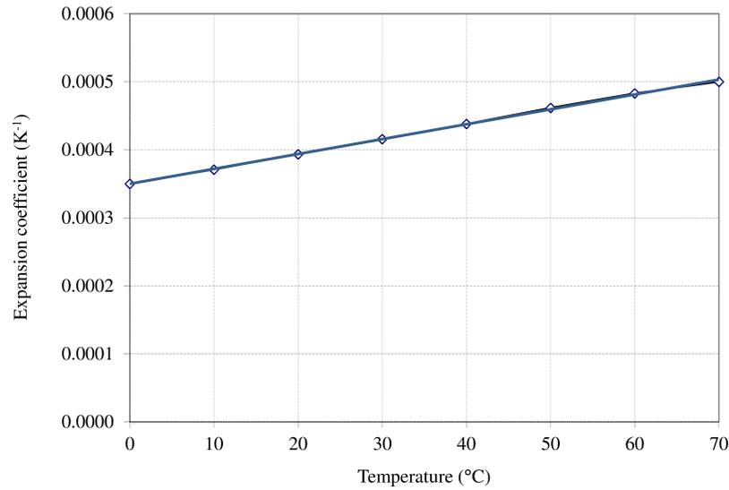
FIGURE 2. Dependence of the volume expansion coefficient of the 30% sugar solution on temperature.
