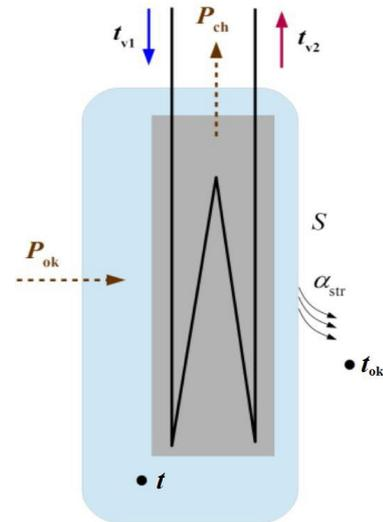
FIGURE 6. Stum tank scheme with thermal flows.
