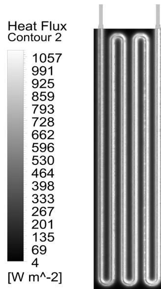
FIGURE 4. Heat flux at  $\Delta t_N = -8^\circ\text{C}$ .
