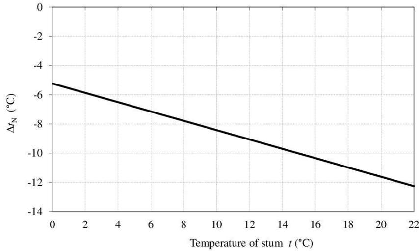
FIGURE 8. Dependence of excessive cooling of the cooling mixture on the stum temperature.
