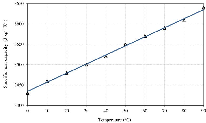
FIGURE 1. Dependence of the specific thermal capacity of the 30 % sugar solution on the temperature.
