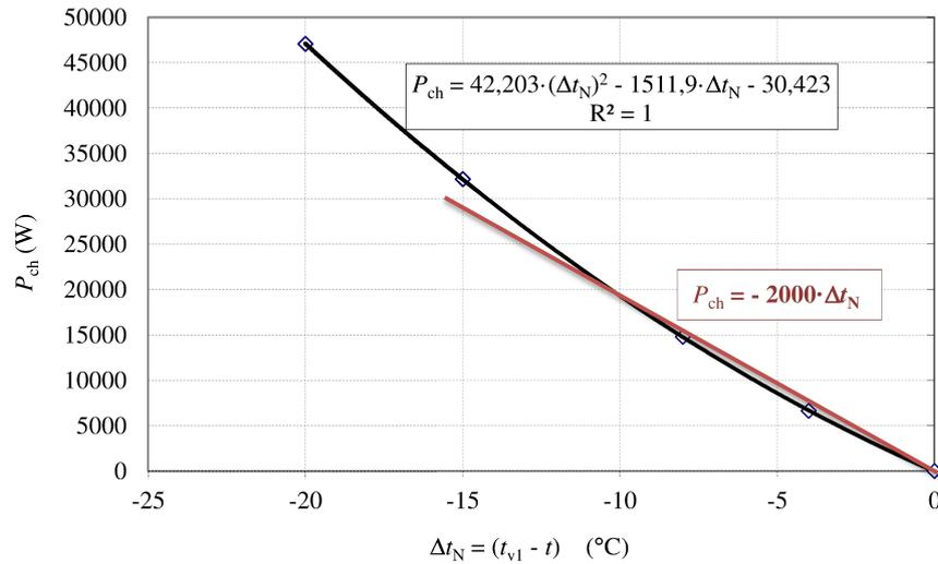
FIGURE 5. Dependence of the cooling performance on the temperatures of the cooling mixture and of the stum.
