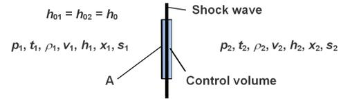
FIGURE 2. Scheme of a shock wave, control volume, and parameters on a normal shock wave in steam.
