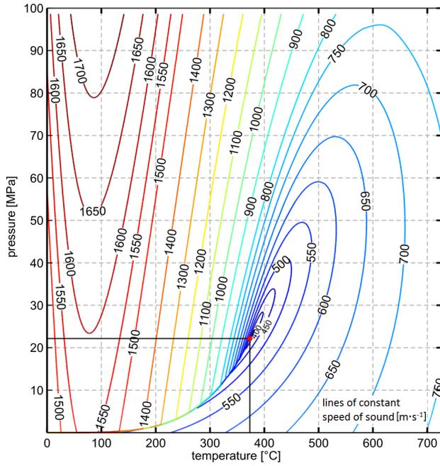
FIGURE 1. Values for the speed of sound [m s<sup>-1</sup>] in water and in steam in a *p*-*t* diagram.
