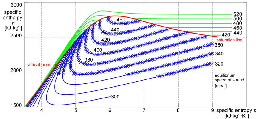
FIGURE 3. The  $h-s$  diagram of water and steam with curves of the constant speed of sound in steam  $a$  [ $\text{m}\cdot\text{s}^{-1}$ ]. The wet steam region blue lines, are from definition (1) and the blue cross values are calculated by means of the model for normal shock waves. Superheated steam  $a$  values according to IAPWS-IF97 are depicted by green curves.
