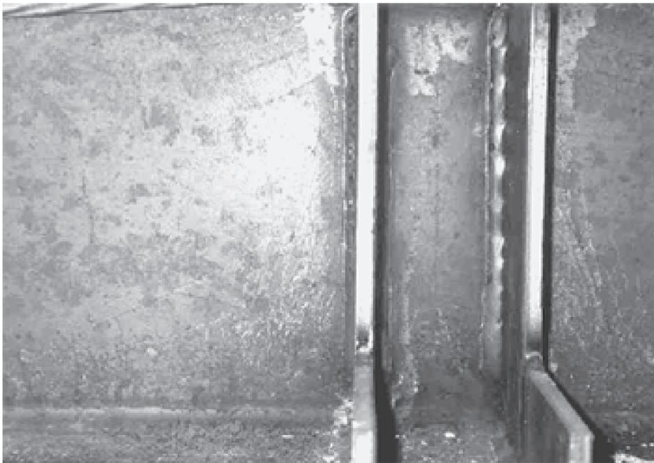
Fig. 7: Diagonal flaking of mill scale indicating the yield development about the inner support section
