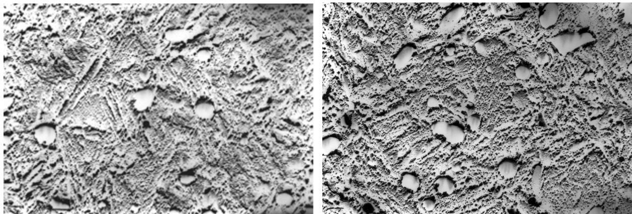
FIGURE 9. Steel for roller bearings 14109.4, 10000 $\times$ , roller-burnished by a working force of 2500 N: (left) a replica at a depth of 0.2mm below the roller-burnished surface; (right) a replica 0.01 mm below the roller-burnished surface.
