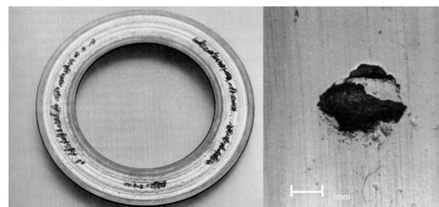
FIGURE 1. Pitting on a bearing ring.
