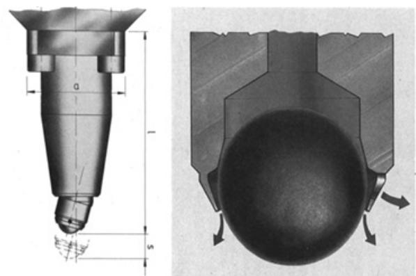
FIGURE 2. The HEGENSCHEIDT hydrostatic roller burnishing tool [11].
