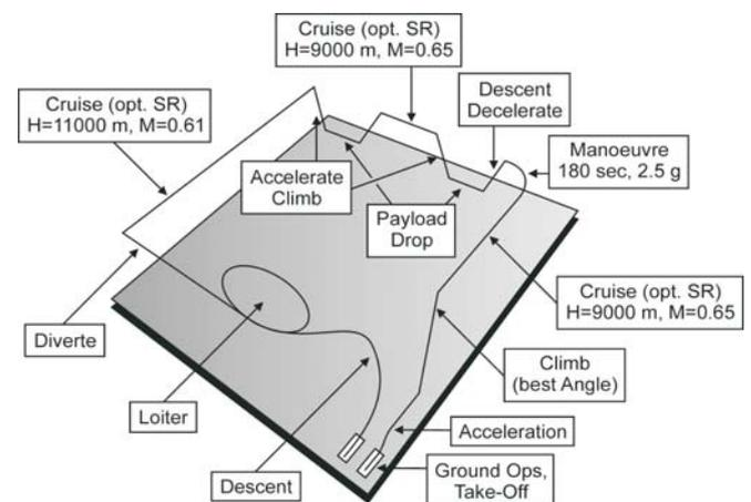
Fig. 3: Flexible mission model (supply mission example)
