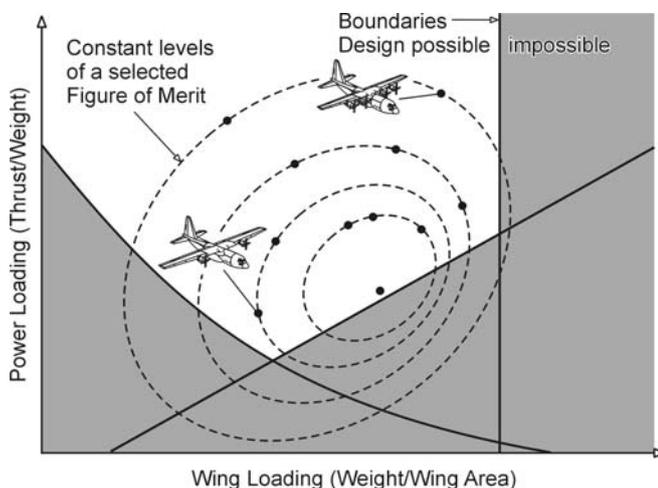
Fig. 4: Design diagram with plottings of evaluable solutions
