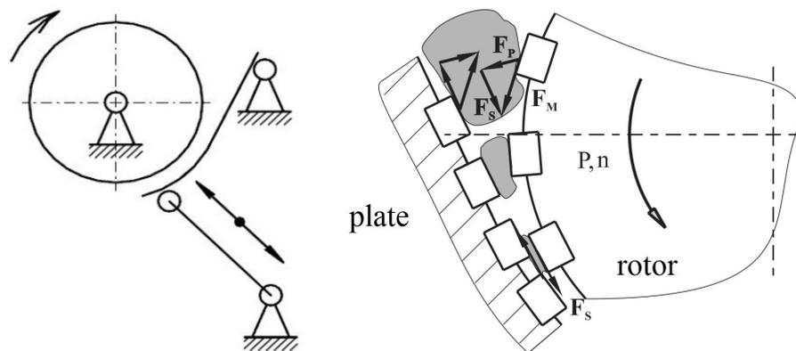
FIGURE 1. The principle of particle disintegration in a retting mill: scheme of the grinding system (left) [18], impact of the forces on a particle (right).
