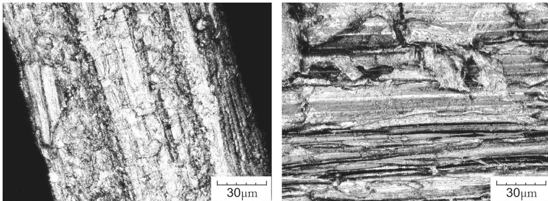
FIGURE 4. Microstructure of wheat straw: A) before disintegration, B) after disintegration.
