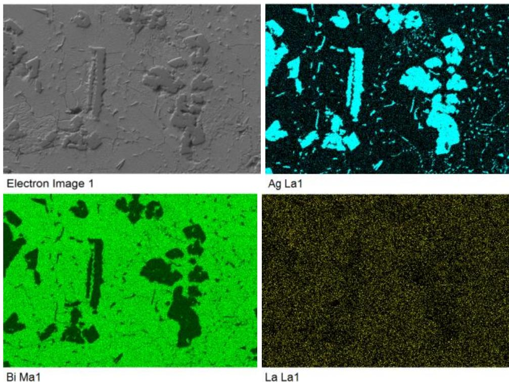
FIGURE 4. Planar analysis of Bi<sub>11</sub>Ag<sub>2</sub>La solder.
