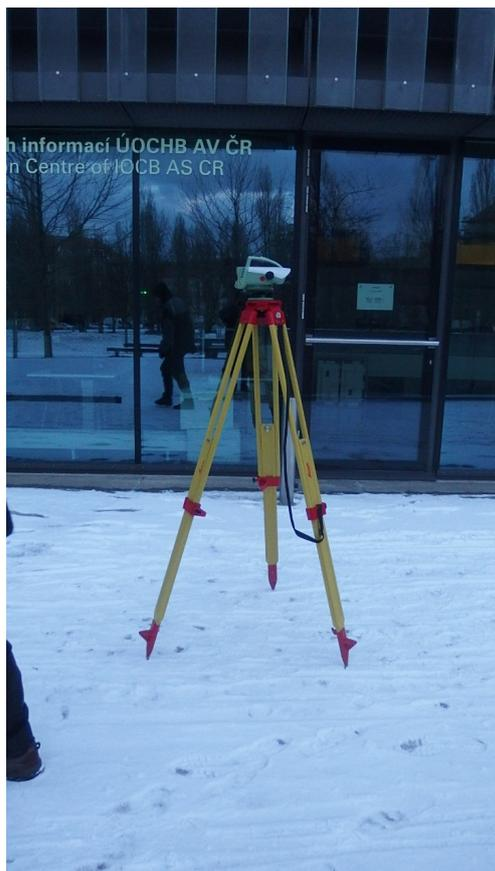
FIGURE 3. DNA 03 levelling instrument; measurement on 8 February 2015
