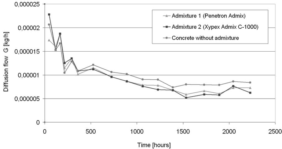
FIGURE 8. Diffusion flow of water vapor through the specimens during the test.
