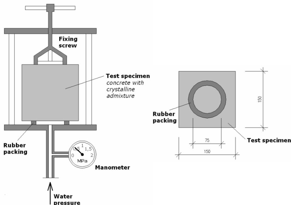
FIGURE 2. The test arrangement.
