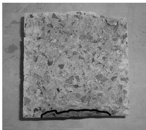
FIGURE 3. A broken test specimen with a visible boundary of seepage.
