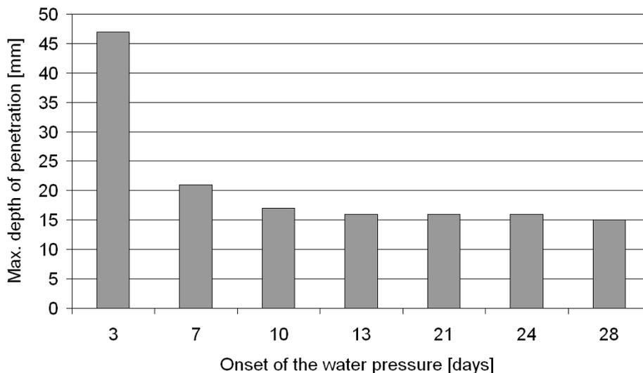
FIGURE 5. Relation between seepage and loading time.
