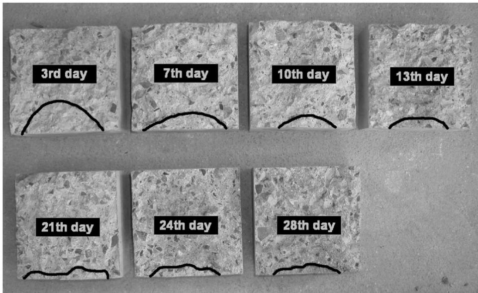
FIGURE 4. The seepage shape in various time periods after the creation of specimens.
