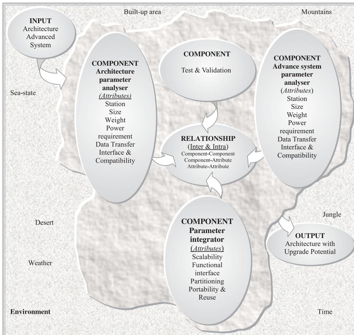
Fig. 1: System structure of an avionics upgrade system
