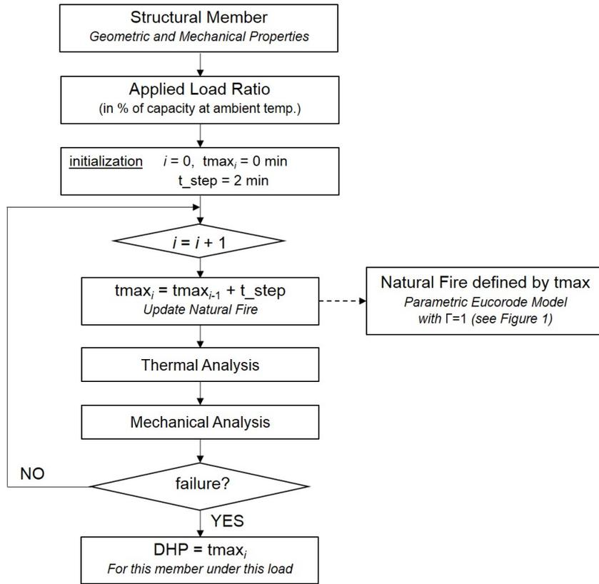
FIGURE 6. Flowchart to obtain the DHP of a member – fixed load ratio method.
