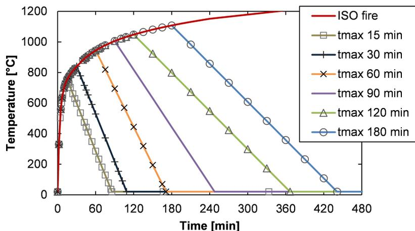
FIGURE 1. Eurocode Parametric Fire Model for Natural Fire.
