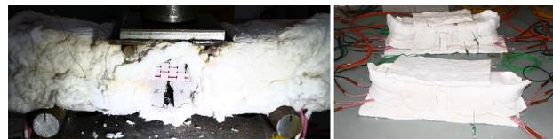
FIGURE 11. Prism specimens during testing (left) and heating (right) process.
