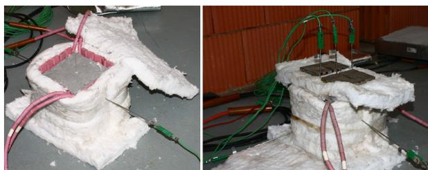
FIGURE 2. Testing setup of pilot cube aiming to observe temperatures inside a cube.
