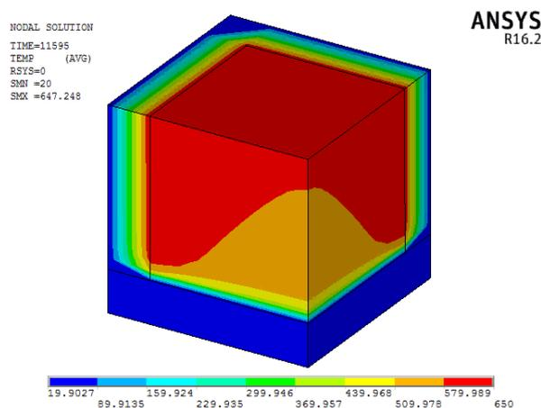
FIGURE 6. Distribution of temperature in simulation, at 193.25 min. A quarter view.
