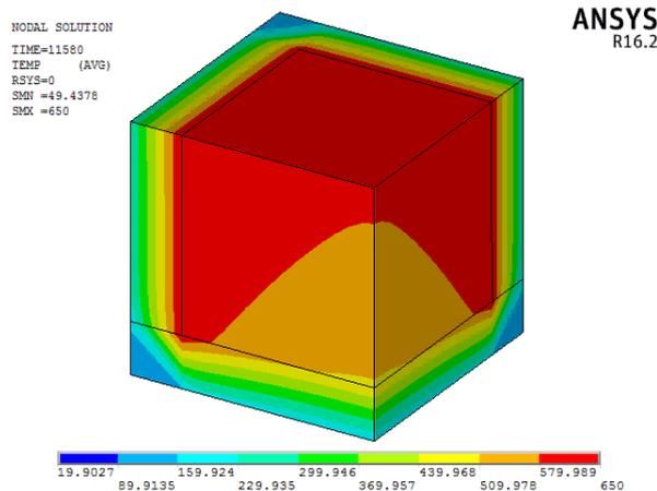
FIGURE 5. Distribution of temperature in simulation, at 193 min. A quarter view.
