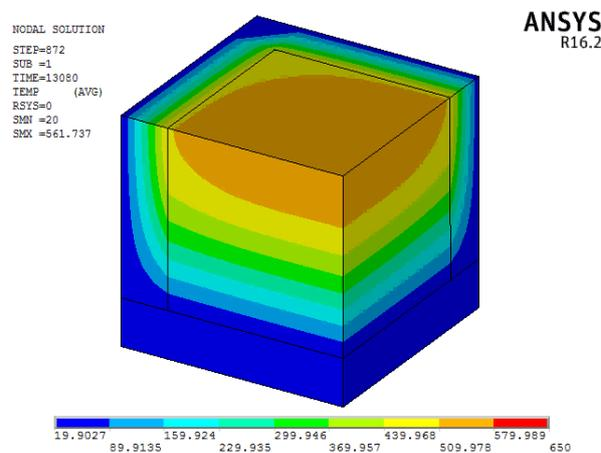
FIGURE 7. Distribution of temperature in simulation, at 208 min. A quarter view.
