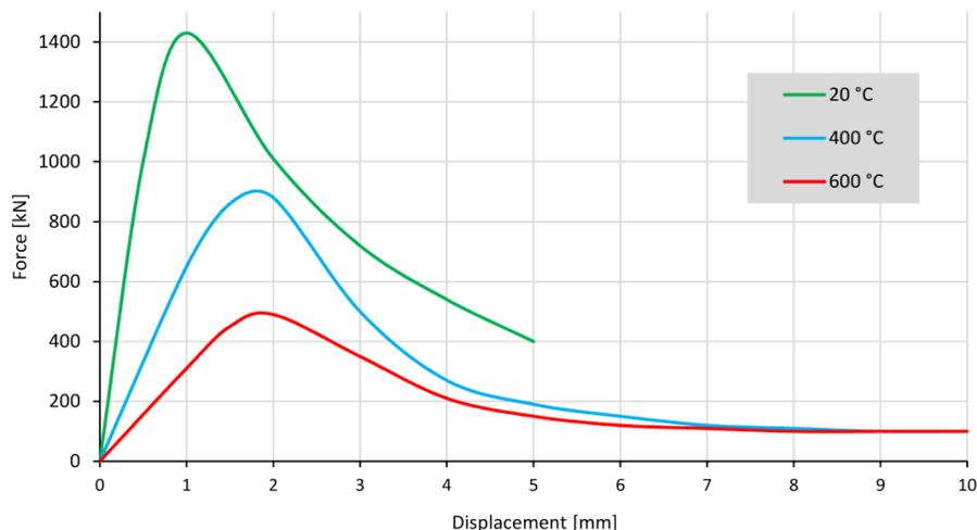
FIGURE 8. Force-displacement diagrams of the concrete specimens in compression.
