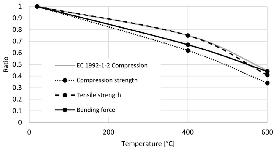
FIGURE 13. The dependence of the compression, splitting tensile strength and bending force on the concrete temperature.
