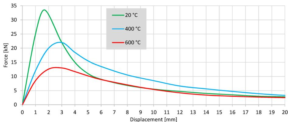
FIGURE 12. Force-displacement diagrams of concrete prisms in four point bending.
