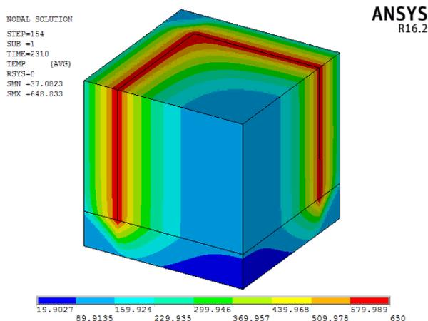
FIGURE 4. Distribution of temperature in simulation, at 39 min. A quarter view.
