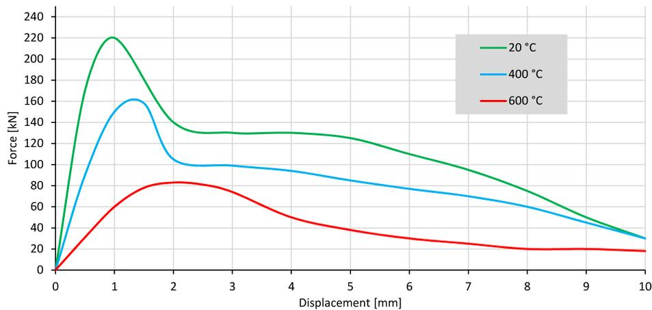
FIGURE 9. Force-displacement diagrams of concrete specimens in split tension.
