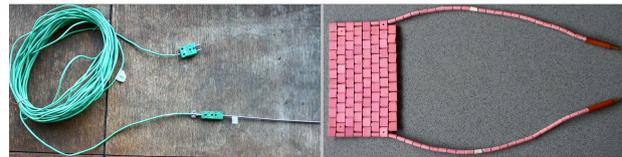
FIGURE 1. K-type thermocouple and ceramic heater.
