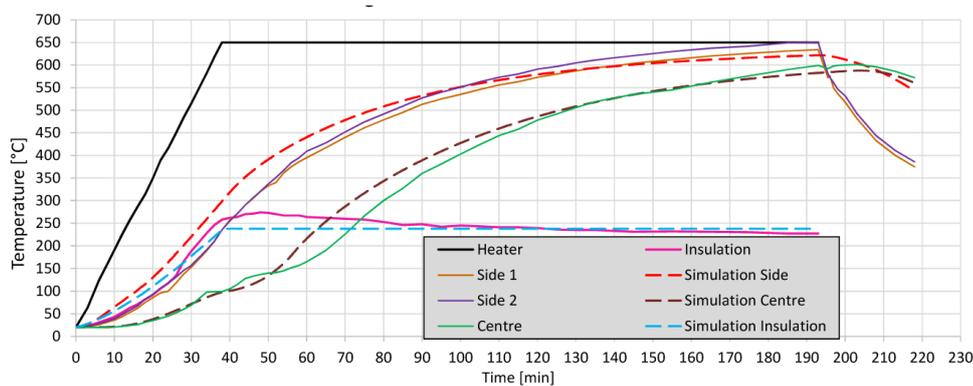
FIGURE 3. Heat transport during heating process.
