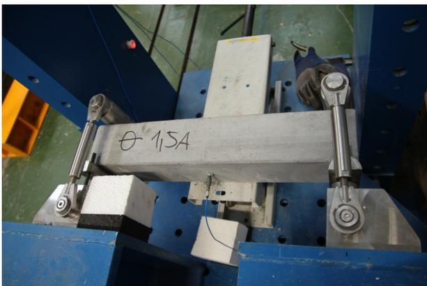
FIGURE 3. The HPCFRC sample fixed in the horizontal impact machine.
