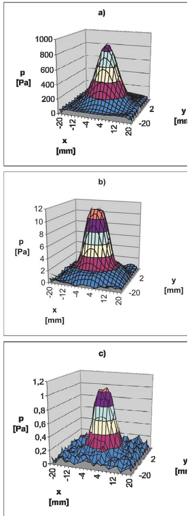
Fig. 3: Microphone measured acoustic field distribution in the  $x$ - $y$  plane at distance  $z = 6.5$  mm from the buffer K with 60 % power from the generator:
