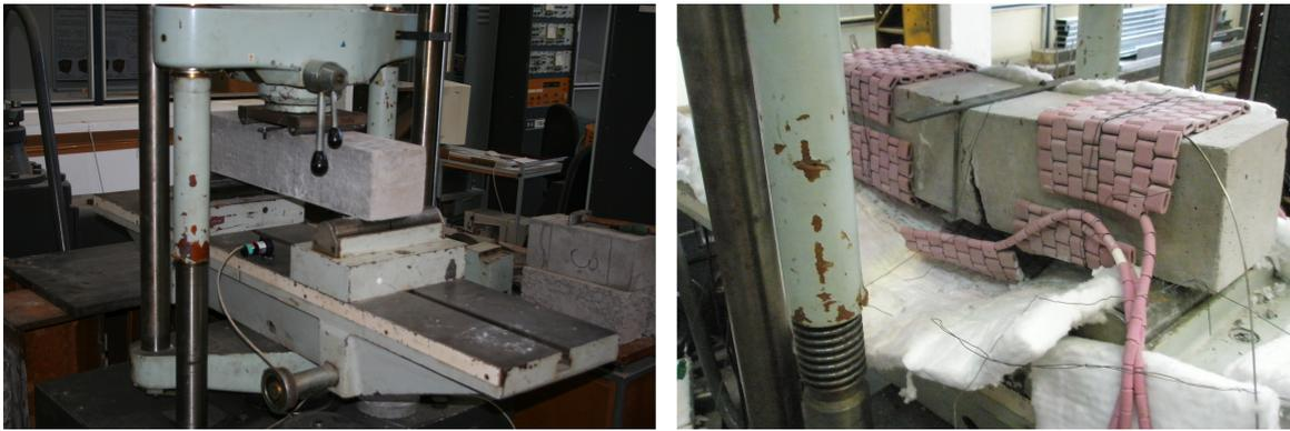
FIGURE 7. Prism during four-point bending test at ambient temperature (left), prism after four-point bending test at elevated temperature (right).
