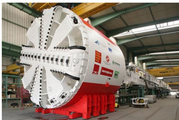
FIGURE 2. EPB shield for Prague metro V.A manufactured in Germany.
