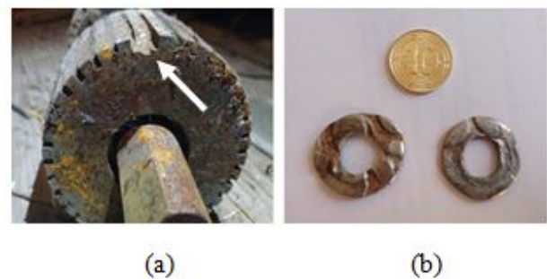
FIGURE 4. (a) Broken roller teeth. (b) Deformed washers that got into the press.
