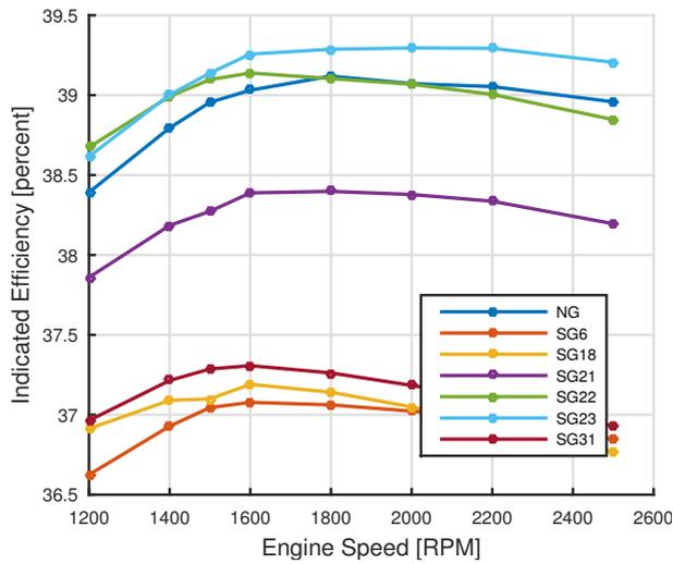
FIGURE 10. Indicated Efficiency comparison of the 6 SGs with the NG fuel for the LGW 702 engine.
