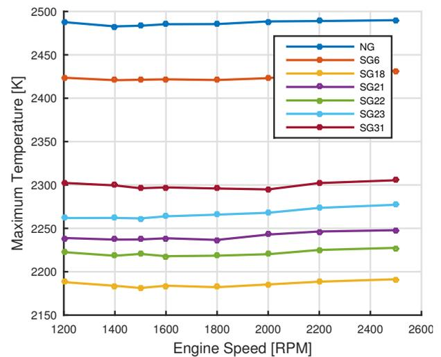
FIGURE 13. Maximum Cycle Temperature comparison of the 6 SGs with the NG fuel for the LGW 702 engine.
