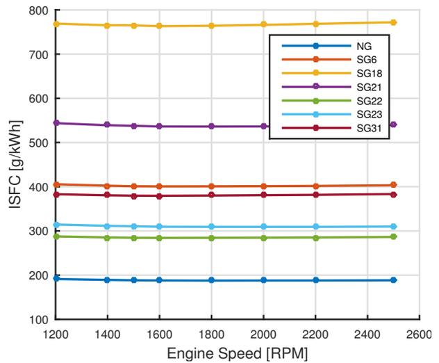
FIGURE 9. ISFC comparison of the 6 SGs with the NG fuel for the LGW 702 engine.
