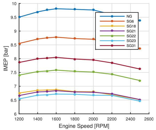
FIGURE 8. IMEP comparison of the 6 SGs with the NG fuel for the LGW 702 engine.
