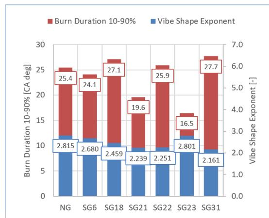
FIGURE 5. *Burn Duration* 10–90% and SI Vibe Burn Exponent comparison of the 6 SGs with the NG fuel for the LGW 702 engine single-cylinder combustion analysis.
