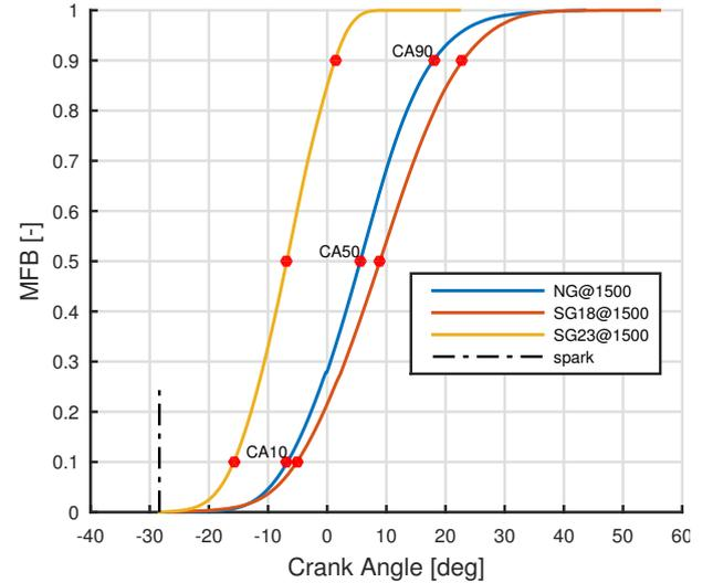
FIGURE 1. Vibe curves and significant burning points for different fuel mixtures at constant spark advance and engine speed.
