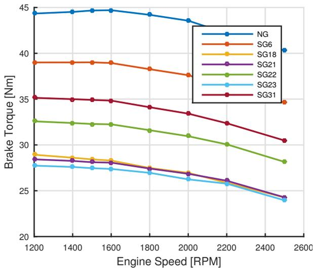
FIGURE 11. Brake torque comparison of 6 SGs with NG fuel for LGW 702 engine.
