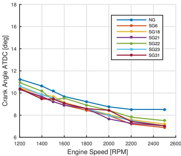
FIGURE 7. Burn duration 10-90 % MFB comparison of the 6 SGs with the NG fuel for the LGW 702 engine.
