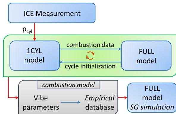
FIGURE 4. Schematic simulation procedure of a new syngas fuel mixture.
