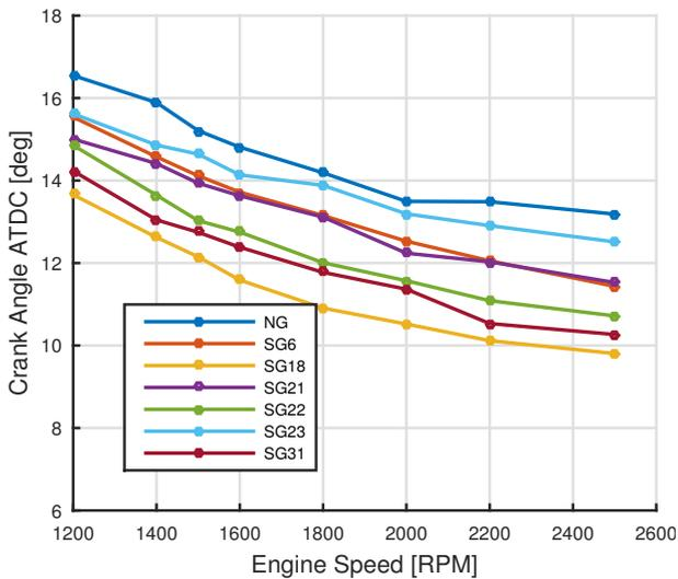
FIGURE 14. Maximum cycle pressure position comparison of the 6 SGs with the NG fuel for the LGW 702 engine.
