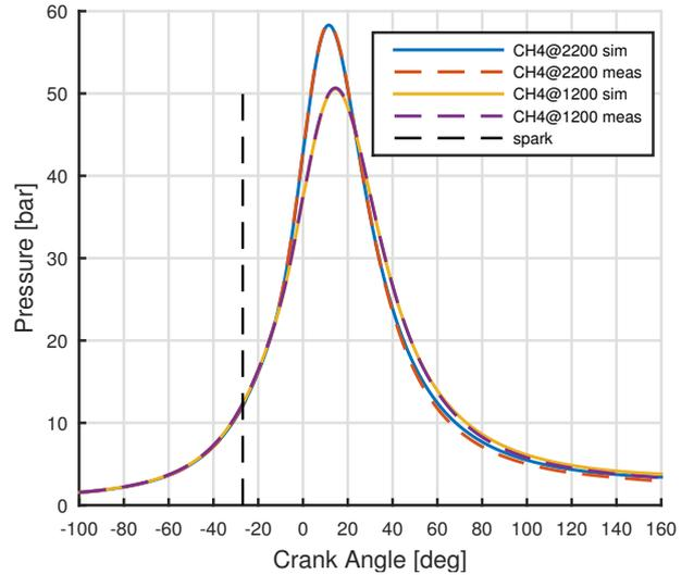
FIGURE 3. Comparison of measured and simulated pressure curves for the optimal solution.
