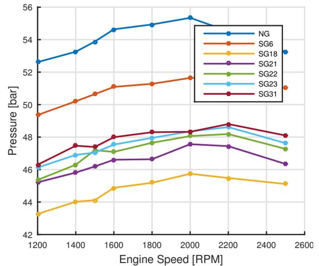
FIGURE 12. Maximum Cycle Pressures comparison of the 6 SGs with the NG fuel for the LGW 702 engine.
