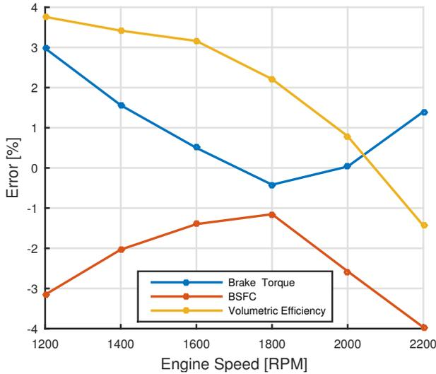
FIGURE 2. Errors on brake torque, the BSFC and volumetric efficiency prediction after first step calibration (simulation – measurement).
