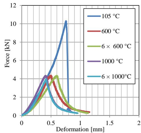
FIGURE 4. Load-deflection diagrams of slabs with 0.25% of fibres.
