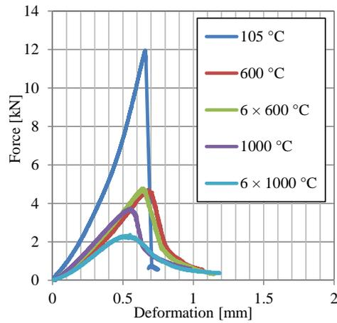
FIGURE 5. Load-deflection diagrams of slabs with 0.50% of fibres.
