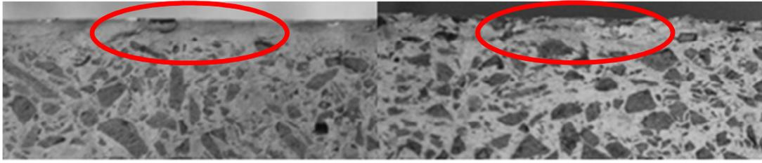
FIGURE 1. Specimen with segregation of fine fraction (0.25 % of fibres – left side) and without segregation of fine fraction (1.00 % of fibres – right side).
