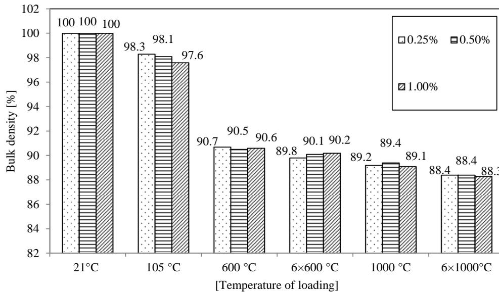
FIGURE 8. Evaluation of bulk density.
