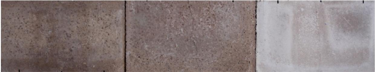
FIGURE 9. Colour changes of tested slabs after the action of elevated temperatures (from the left side: 105 °C, 600 °C, 1000 °C).
