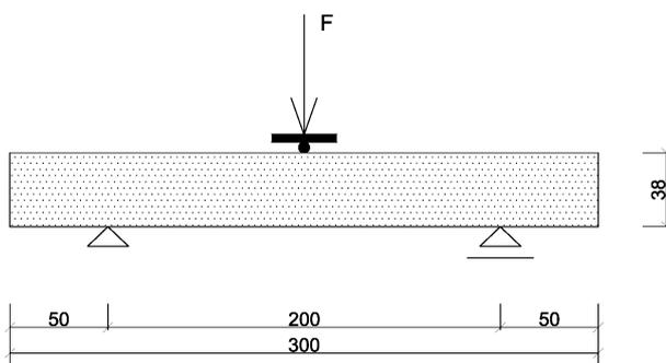
FIGURE 3. Slab bending test arrangement [mm].
