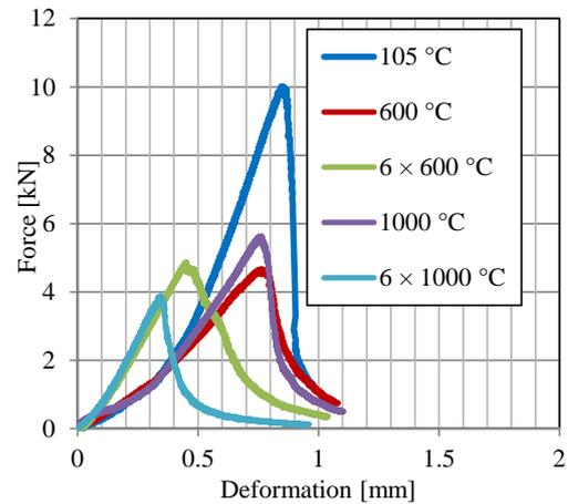
FIGURE 6. Load-deflection diagrams of slabs with 1.00% of fibres.
