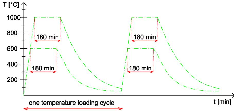
FIGURE 2. Description of thermal loading cycles.
