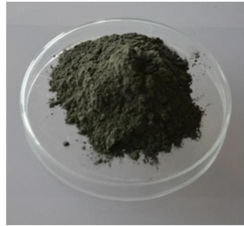
FIGURE 2. Dust from brake lining production.
