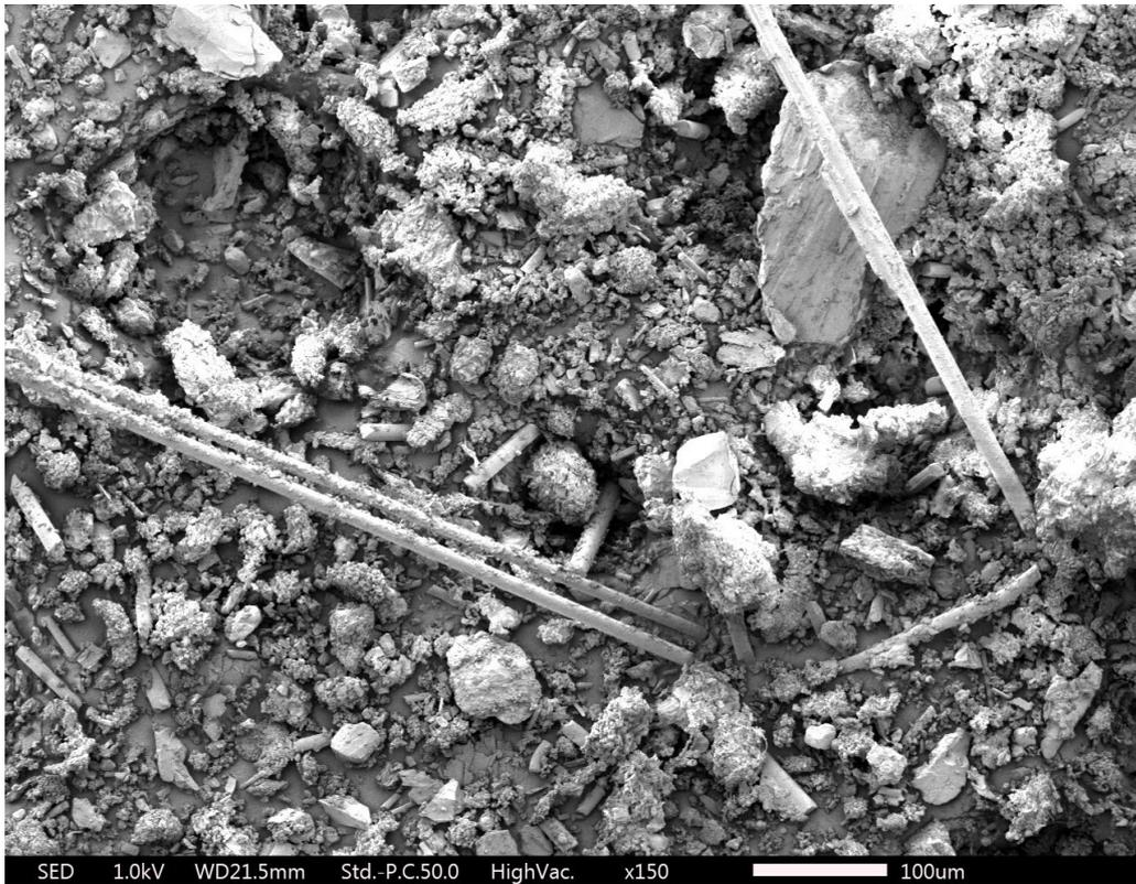
FIGURE 14. Shot of brake powder at 150-times enlargement, made by a JoelR Scanning electron microscope (SED-1.0kV-WD21.5mm-Std.P.C.50.0-HighVac-x150).
