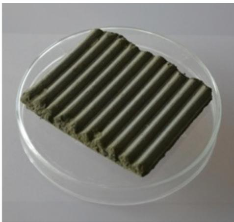
FIGURE 5. Profiled strip of experimental material from compacting process.
