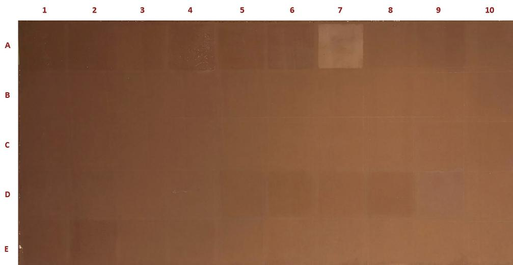
FIGURE 2. Condition after application of all consolidants on one of the test panels.
