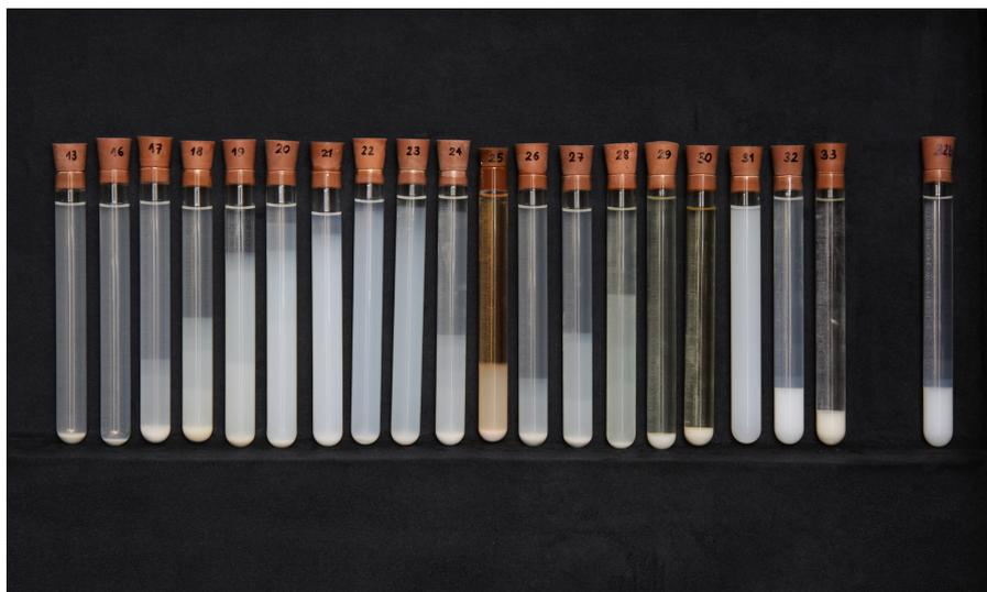
FIGURE 1. Sedimentation process of selected consolidants over 57 days. Test tubes 13, 16 and 17 contain lime suspensions diluted to 5 g/l, test tubes 28–33 contain lime suspensions mixed with silicic acid esters.
