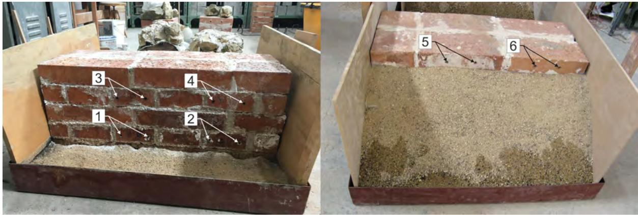
FIGURE 6. Placement of measuring points in masonry (on the laboratory model).
