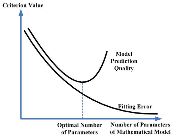
FIGURE 15. Typical model prediction and fitting properties as a function of its number of parameters.
