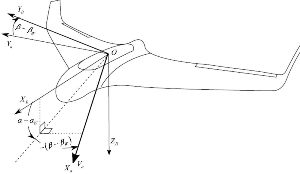
FIGURE 4. Body-axis and wind-axis reference frames of the UAV.
