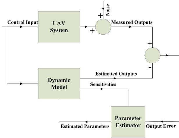
FIGURE 5. Block diagram for the output-error parameter estimator.
