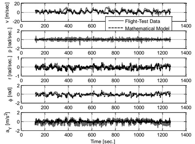
FIGURE 16. Prediction capability of the model with estimated parameters for the OEM-AIV (with initial condition from analytical aerodynamic parameters of SX8FW case) and for additional flight-test data.
