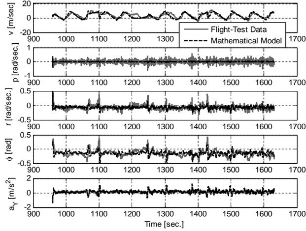
FIGURE 10. Flight data and responses of the model with the OEM-IAV parameters with initial condition from analytical aerodynamic parameters of SX8FW.
