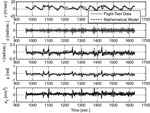
FIGURE 11. Flight data and responses of the model with the LSM-OEM-AC parameters.
