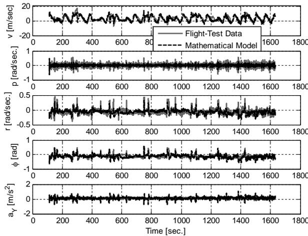
FIGURE 14. Flight data and responses of the model with the OEM-IAV parameters with initial condition from analytical aerodynamic parameters of the ZFW.
