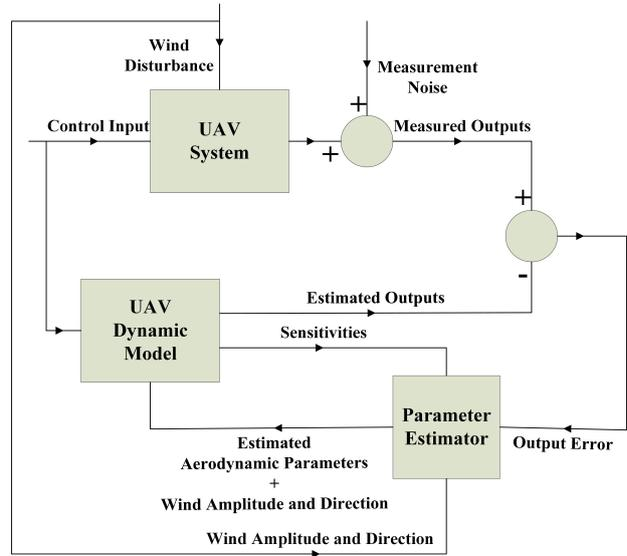
FIGURE 6. Block diagram for the output-error parameter estimator with wind estimation.
