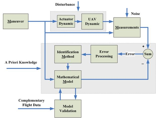
FIGURE 7. Identification of the UAV and actuator dynamic model.
