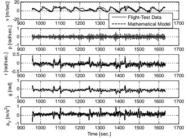
FIGURE 12. Flight data and responses of the model with the OEM-MC parameters.
