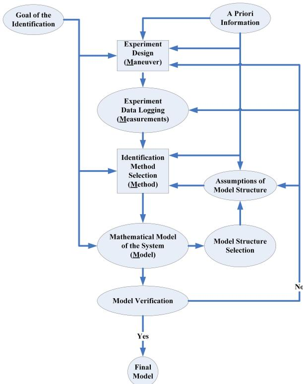
FIGURE 1. Quad-M principles for flight system identification.
