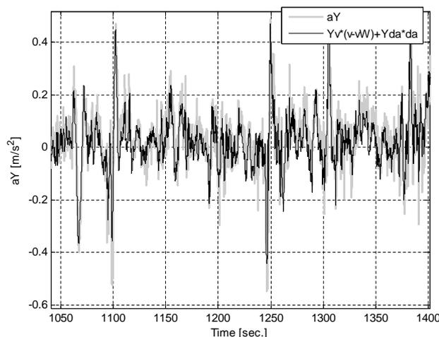
FIGURE 9. Part of the time history match of the lateral acceleration and its regressor prediction.
