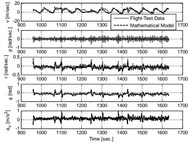
FIGURE 13. Flight data and responses of the model with the LSM-OEM-MC parameters.
