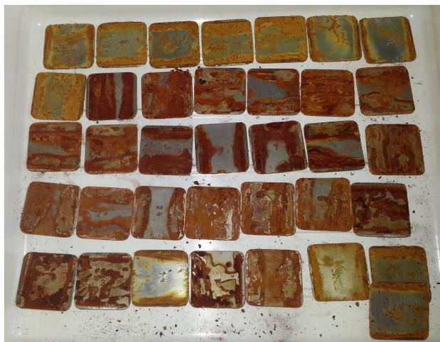
FIGURE 5. Coupons before staining in hydrochloric acid
