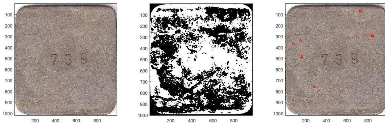
FIGURE 8. Graphic evaluation of the corrosion coupon using the Matlab software – coupon 739a. Areas evaluated as pitting corrosion are marked with a red colour
