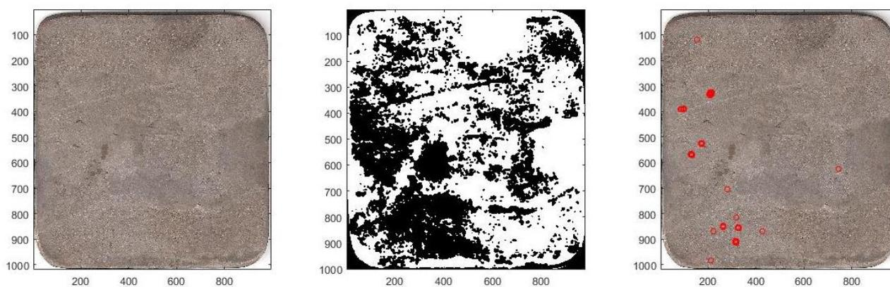
FIGURE 9. Graphical evaluation of the corrosion coupon using the Matlab — coupon 739b
