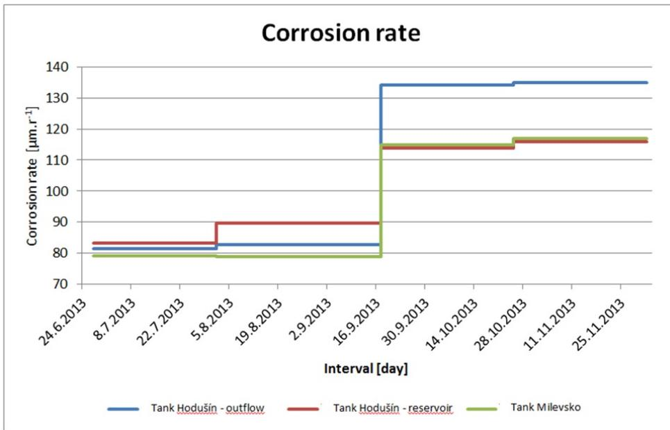
FIGURE 7. Corrosion rate evaluations according to consecutive intervals — June 25th–September 17 2013 (0–82 days) and September 17th–December 2nd 2013 (0–76 days)
