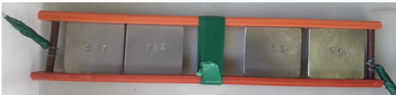
FIGURE 1. Four testing plates mounted in a holder and prepared to be put into the pipeline
