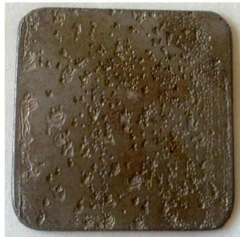
FIGURE 6. Coupon after exposure
