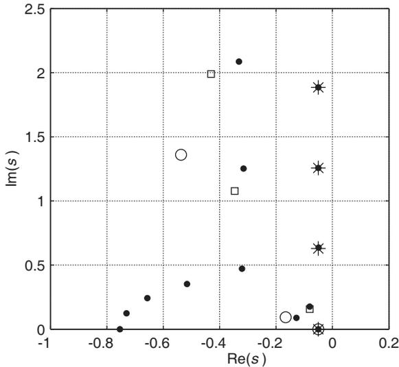
Fig. 7: Spectra of closed loop system for  $T_f = 10$  and  $\eta_f = 7$ , detail of Fig. 9
