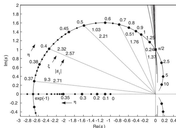
Fig. 1: The trajectory of the dominant couple of roots of the characteristic function  $M(s) = 1 + \exp(-s\eta)$  with respect to  $\eta$ ,  $\xi = |\beta|/\omega$ ,  $s_{1,2} = \beta \pm j\omega$  (the time constant  $T$  is considered here as a time-scale unit)
