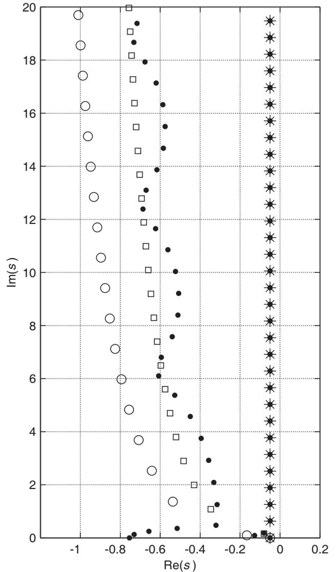
Fig. 9: Spectra of closed loop system for  $T_f = 10$  and  $\eta_f = 7$ . Spectra of closed loop system (19): black circles – poles of (19), empty circles – zeros of (19), asterisks – roots of  $N(s)$ , squares – poles of system (17) (ideal closed loop).
