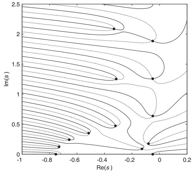
Fig. 6: Poles of the closed loop system with plant model (20) and controller (5),  $\text{Re}(M_{wy}(s)) = 0$  - solid,  $\text{Im}(M_{wy}(s)) = 0$  - dashed,  $M_{wy}(s)$  - given by (21)
