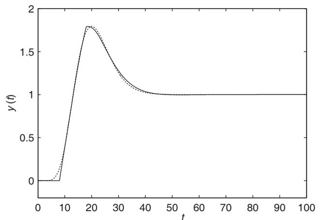
Fig. 4: Step responses of system (20) (dashed) and of its approximation (5) (solid)
