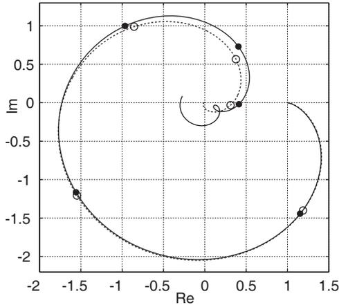
Fig. 5: Frequency responses of system (20) (dashed) and of its approximation (5) (solid)
