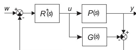
Fig. 2: Internal model control (IMC) scheme
