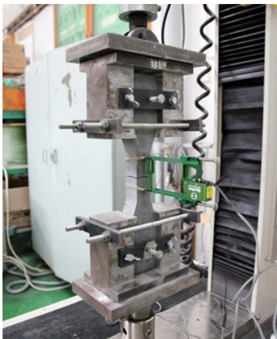
FIGURE 2. Specimen in claws with installed extensimeter.
